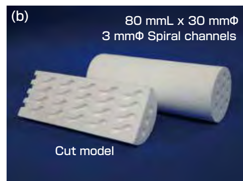
Fig.10 (a) Conventional water-purification ceramic filter has unidirectional straight channels, while the AM techniques enable more complicated channels, e.g. , spiral ones. (b) an alumina filter model produced by PLM, containing spiral channels of 3 mm diameter whose traces are observed in the cut model
