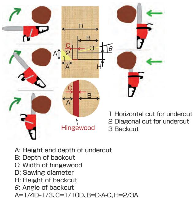
Fig. 13 Cut dimension and order of cuts
