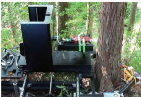
Fig. 10 TATSUMI I: Composed only of rectilinear pair
