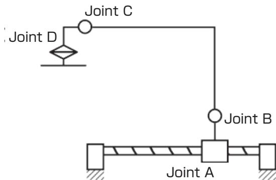
**Fig. 15 Arrangement of degrees of freedom**
