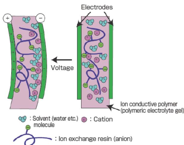
Fig. 1 Schematic diagram of the structure of an ion conductive polymeric actuator and the bending response principle
