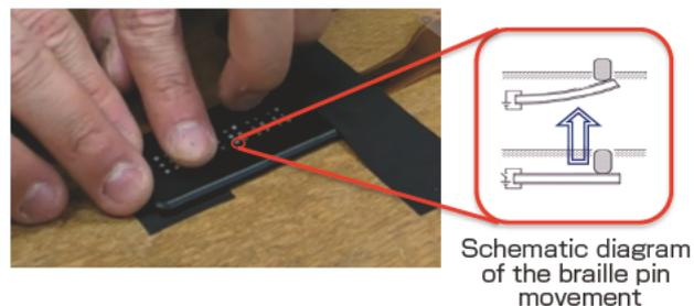
**Fig. 6 Braille display using the bucky gel actuator**
