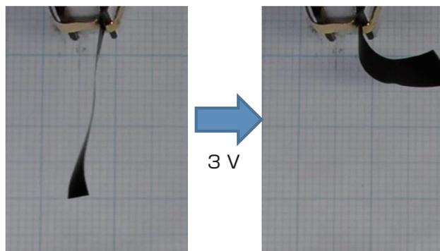
**Fig. 5 Deformation of the bucky gel actuator at 3 V applied voltage**
