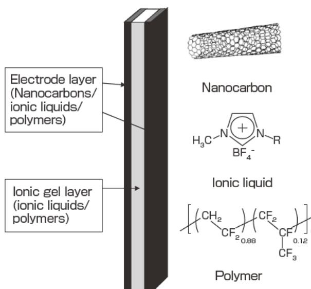
Fig. 3 Schematic diagram of the structure of the bucky gel actuator
