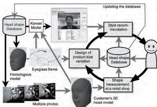
**Fig. 5 A system to produce eyeglass frames according to the “Finding well-fitting products” approach**
