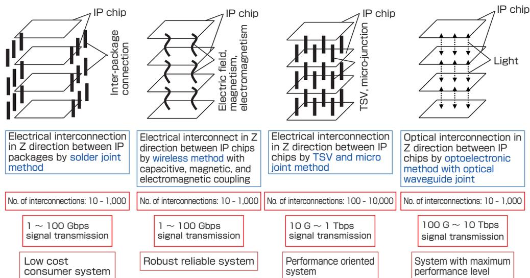
Fig. 2 3D IC chip stacking system technology
