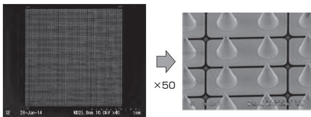
**Fig. 8 SEM photograph of the 10,000 (100 x 100) cone-shaped Au micro-bump array (partially enlarged x50)**
