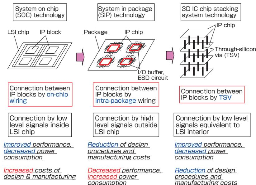
**Fig. 1 Progress of electronic hardware system integration technology**
