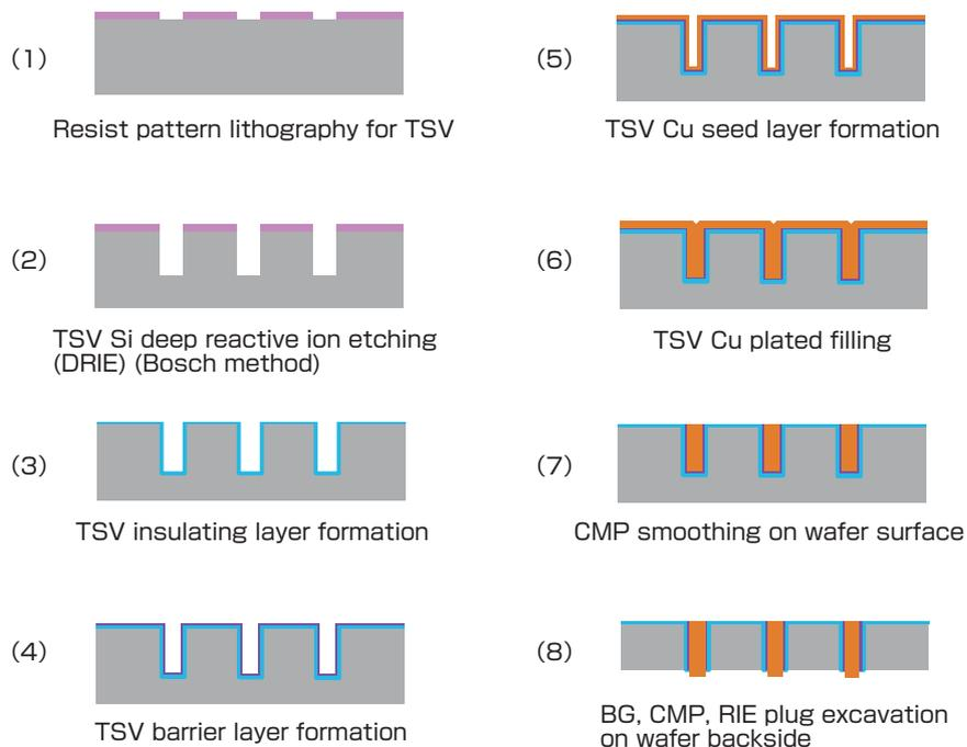
**Fig. 3 Process flow for manufacturing the TSV**
