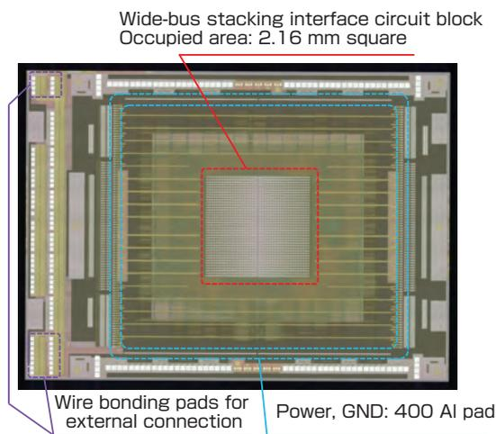
**Fig. 14** Test IC device for Cool Interconnect evaluation
