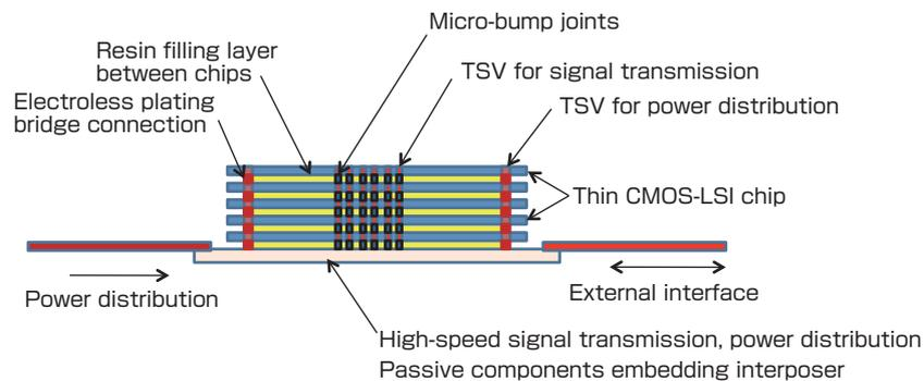
**Fig. 4 Fundamental technologies for the 3D IC chip stacking system integration (stacking process and evaluation test)**
