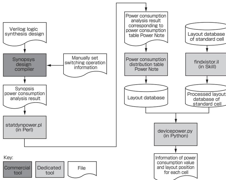
Fig. 11 Flow of design data for the thermal aware IC layout design regarding electrothermal IC design
