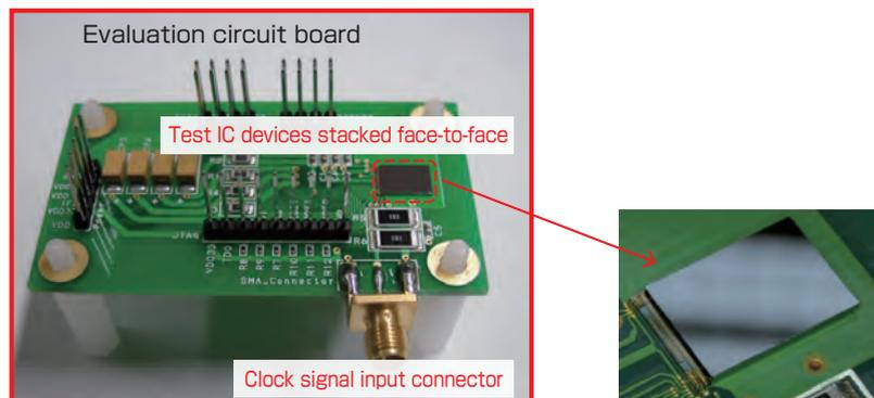
**Fig. 16** Test IC device mounted on the evaluation circuit board after stacking
