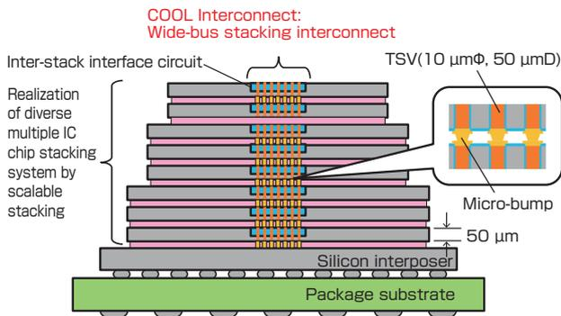
Fig. 12 Conceptual diagram of the Cool Interconnect
