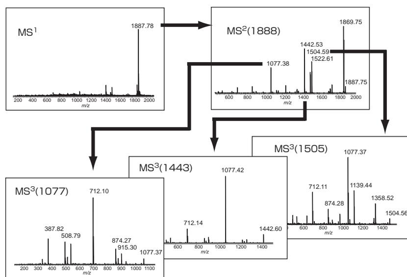
Fig. 6 Tree structure of the multistage MS
