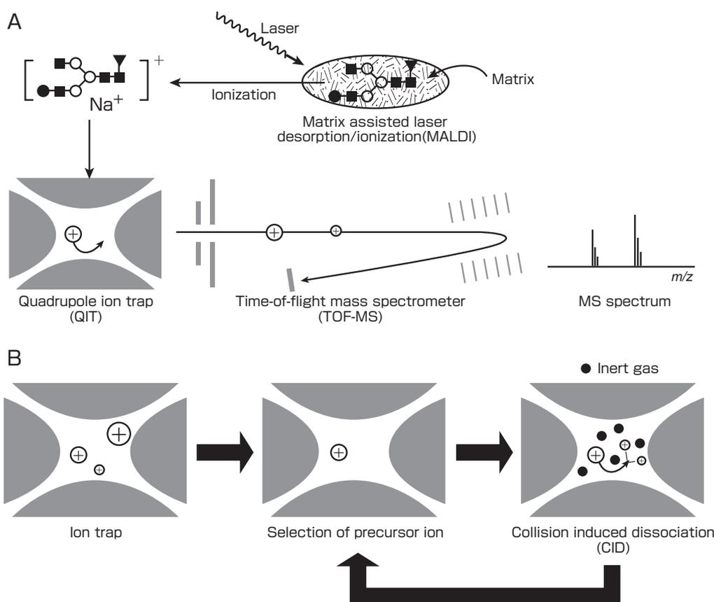
**Fig. 2 Schematic diagram of the MALDI-QIT-TOF MS**
