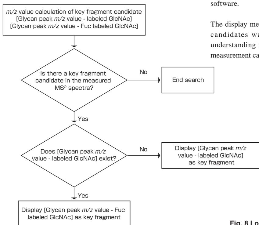
Fig. 8 Logic flow of the key fragment identification
