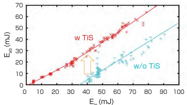
**Fig. 14 Effect of TiS laser on the absorbed energy ( $E_{ab}$ ) of YAG laser vs incident energy of the YAG laser ( $E_{in}$ )**
