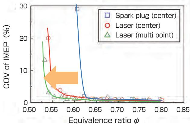
**Fig. 10** Dependence of COV of IMEP on equivalence ratio
