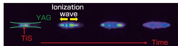
**Fig. 15 Temporal breakdown process with initial electron supply**
