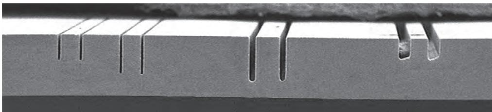
Fig. 13 Cross-sectional SEM photograph of deep groove processing by LIBWE method on aluminosilicate glass substrate (thickness of glass substrate: 0.5 mm). Groove width 20 μm (left), 50 μm (center), and 80 μm (right).
