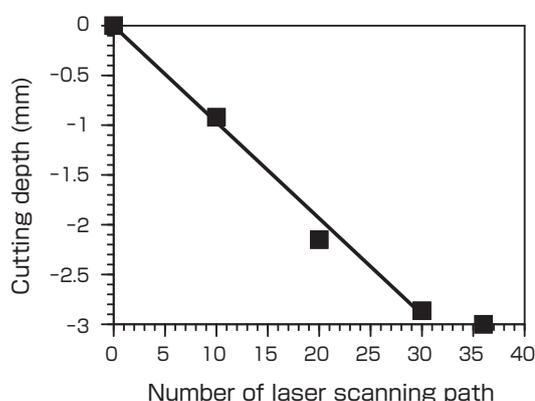
Fig. 5 Cutting depth of 3 mm thick CFRP sample using double-line multipath laser irradiation (Laser beam scanning speed of 3.6 m/s)
