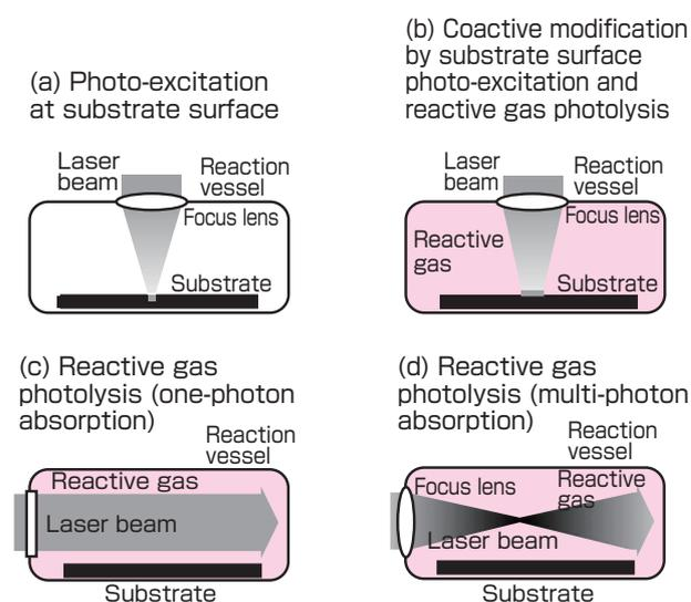
Fig. 2 Surface modification method by laser processing
