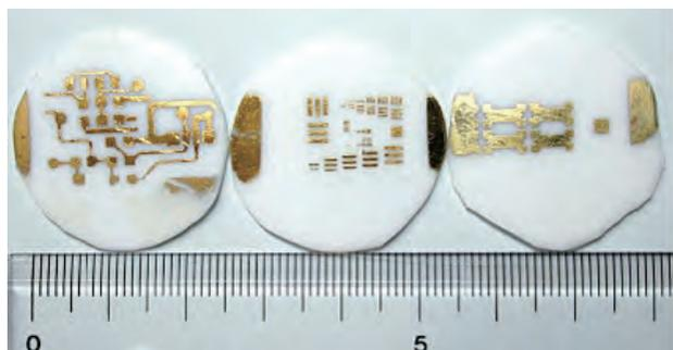
**Fig. 10** Nickel chemical plating on PTFE (Topmost surface of plated film has been gold replaced.)<sup>[12]</sup>
