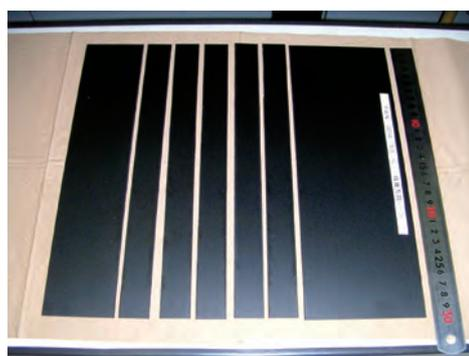
**Fig. 3 Laser cutting of 30 cm square CFRP substrate**
