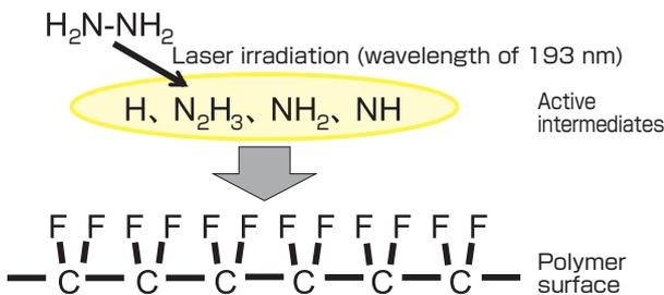
Fig. 7 Schematic diagram of the surface reaction
