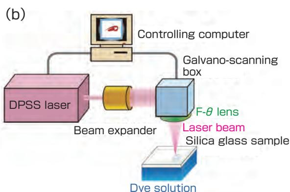
**Fig. 11** Experimental apparatus for the LIBWE method
