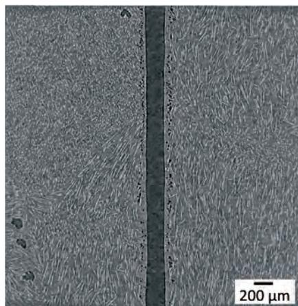
Fig. 4 Cross-sectional picture of micro-X-ray CT of CFRP sample after laser cutting<sup>[8]</sup>
