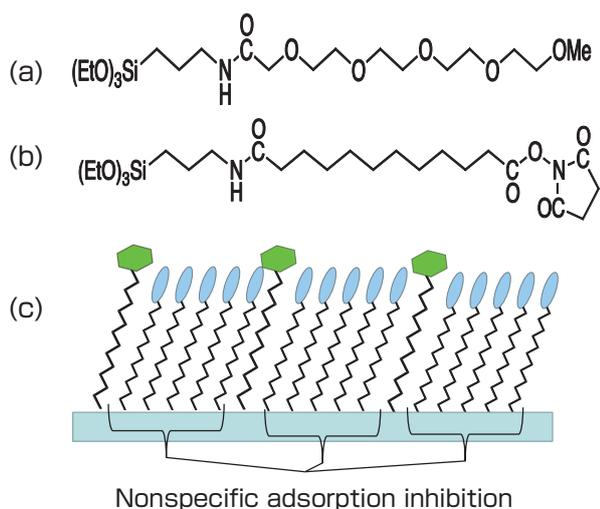
**Fig. 11 Nonspecific adsorption inhibiting surface**
