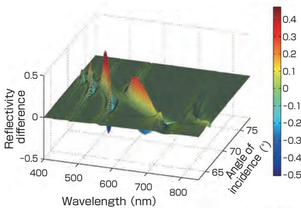
**Fig. 2 Calculation results of the dependence of reflectivity change on angle and wavelength**
