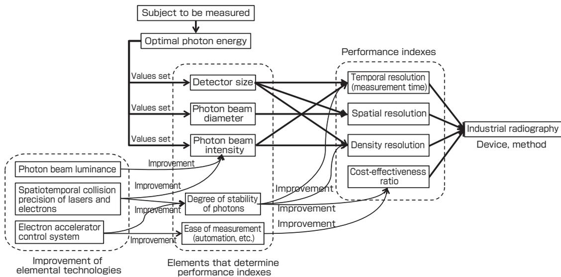
**Fig. 8 Improvement of elemental technologies, elements that determine the performance index, and relationship of the sophistication of devices and methods**
