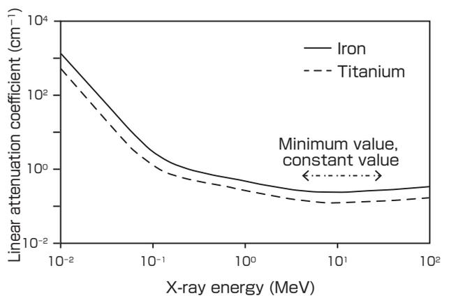
Fig. 2 Linear attenuation coefficients of iron and titanium at 10 keV ~ 100 MeV<sup>[6]</sup>
