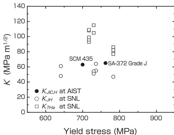
**Fig. 7 Relationship between yield stress and fracture toughness of Cr-Mo low-alloy steel<sup>[18][20]</sup>**
