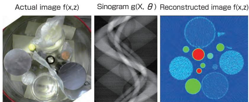
**Fig. 6 (Left) Sample photograph, (center) sinogram, and (right) CT image<sup>[9]</sup>**
