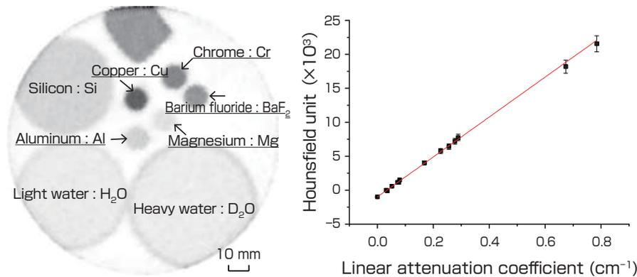
**Fig. 7 (Left) Plot of the linear attenuation coefficients of various materials and the CT values expressed by HU.<sup>[10]</sup> The symbols in the diagram represent the substances, e.g. D<sub>2</sub>O = heavy water.**
