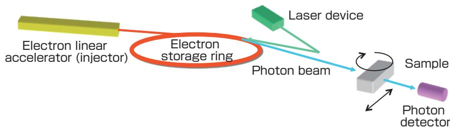
Fig. 4 LCS photon CT system using the electron accelerator
