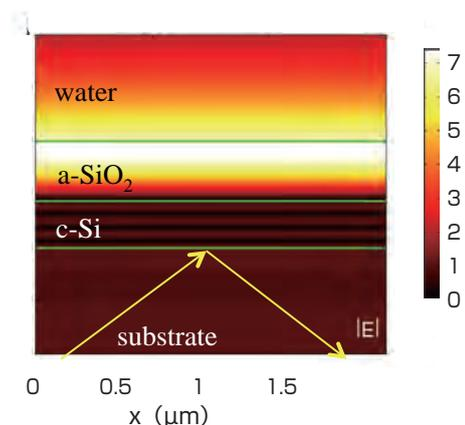
**Fig. 5 Electric field intensity distribution of waveguide modes at 220 nm c-Si layer, 284 nm SiO<sub>2</sub> layer, and 512 nm excitation wavelength**
