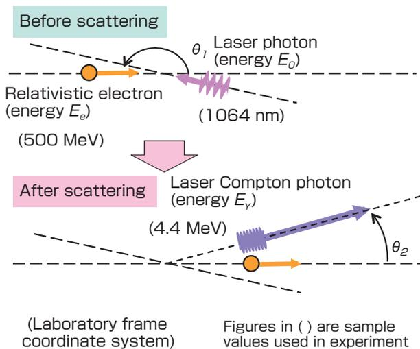
Fig. 1 Kinematics of laser Compton scattering
