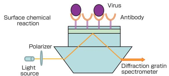
**Fig. 4 Optical arrangement of the waveguide mode sensor**
