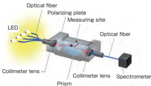
**Fig. 3 Wavelength sweeping waveguide mode sensor**
