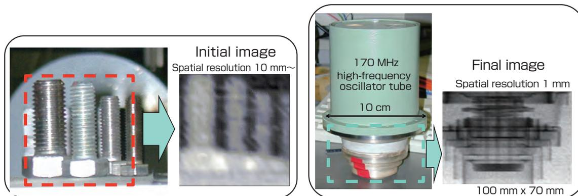
**Fig. 5 Transmission radiography using LCS photons**
