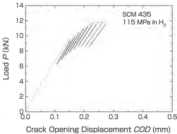
**Fig. 6 P-COD curve of SCM435 by the unloading elastic compliance method**
