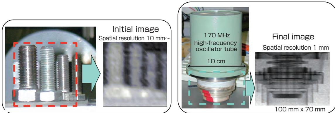
**Fig. 5 Transmission radiography using LCS photons**
