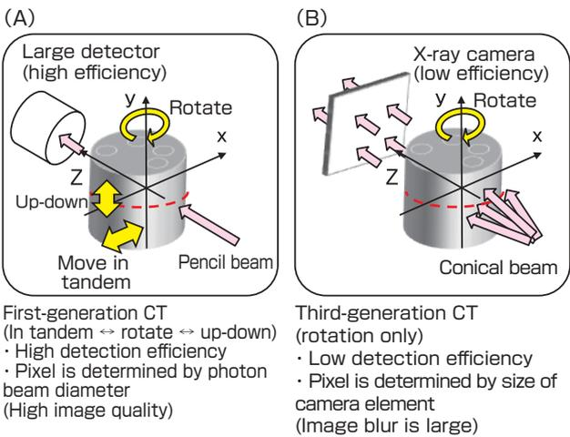
Fig. 3 Explanation of CT generations. (A) First-generation and (B) third-generation.
