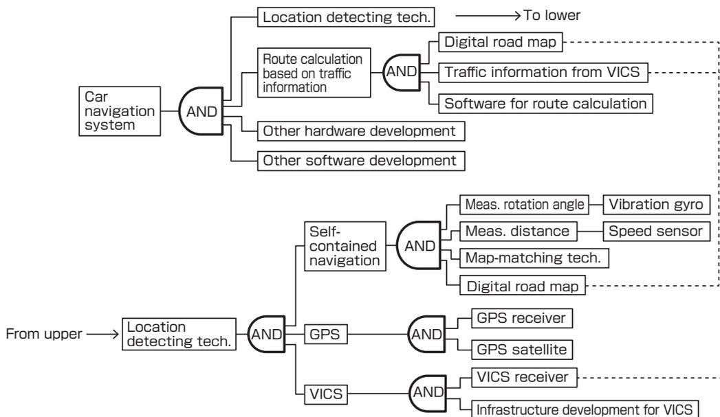
**Fig. 13 Technology architecture of the third generation of car navigation systems**
