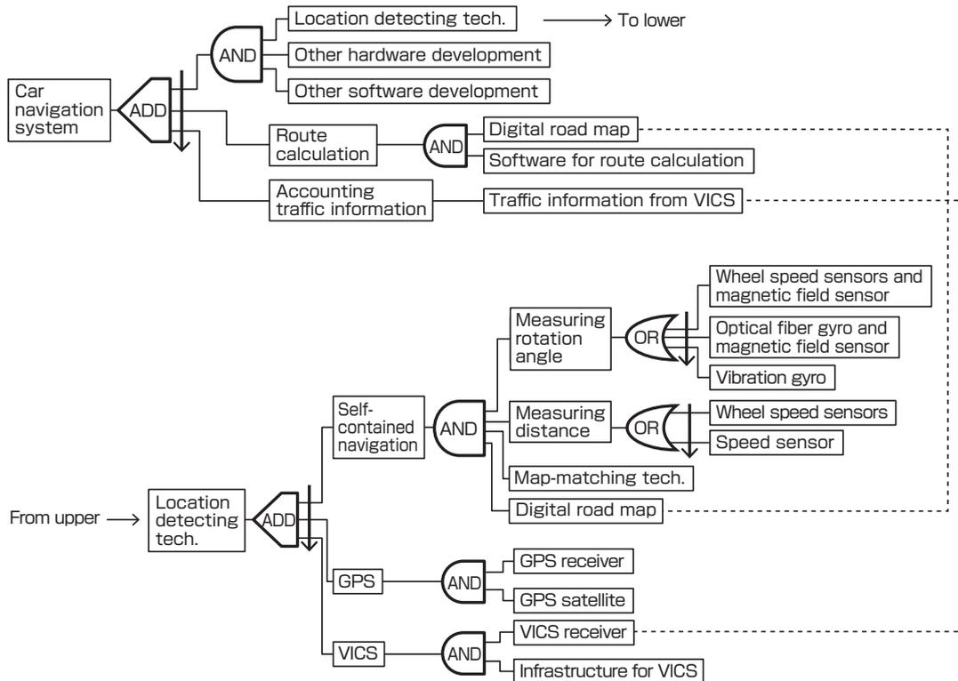
**Fig. 14 Innovations in technology architecture of car navigation systems**
