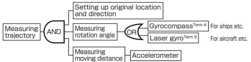
Fig. 5 Former method to measure trajectory by self-contained navigation
