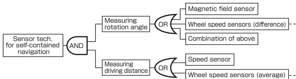
**Fig. 9 The choice for sensor technologies in the first development of a car navigation system**
