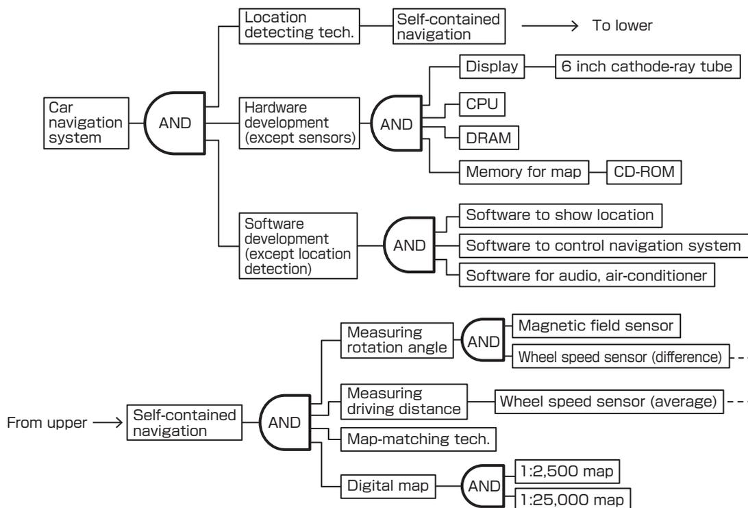
**Fig. 10 Technology architecture when the first car navigation system was finished (1989 model)**
