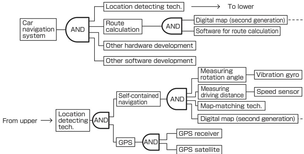
**Fig. 12 Technology architecture of 1992 model (second generation)**
