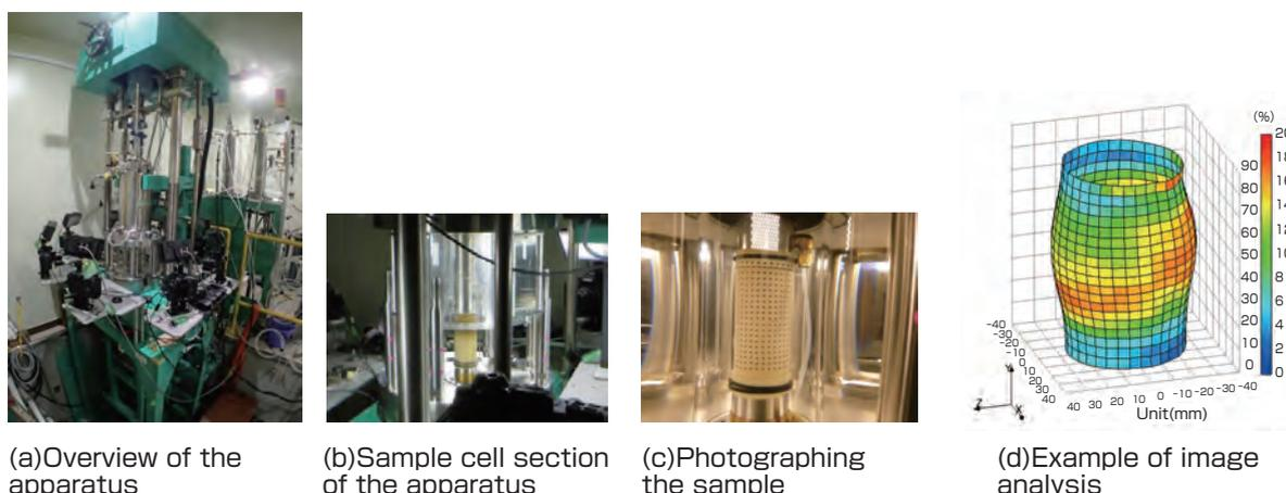
**Photograph 1. Transparent acrylic cell triaxial testing (TACTT) system**
