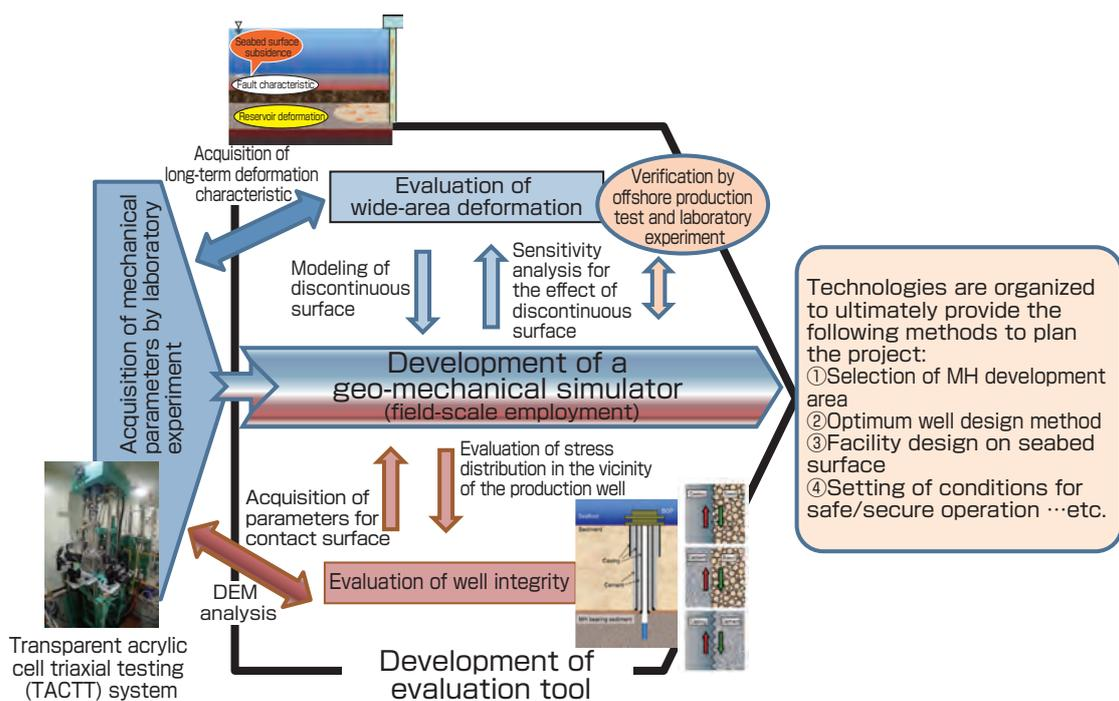
**Fig. 4 Development of evaluation tool for sedimentary characteristics**
