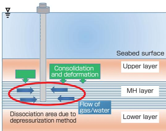
**Fig. 1 Mechanical behavior of the MH layer**
