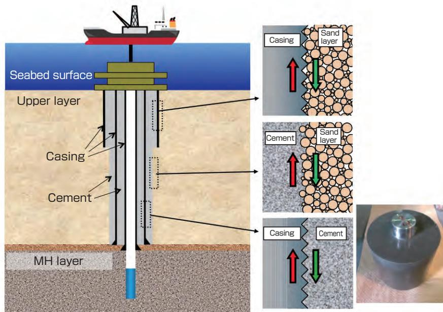
**Photograph 2. Sample for measuring the contact surface strength between the casing and cement (part of the diagram has been modified)<sup>[21]</sup>**
