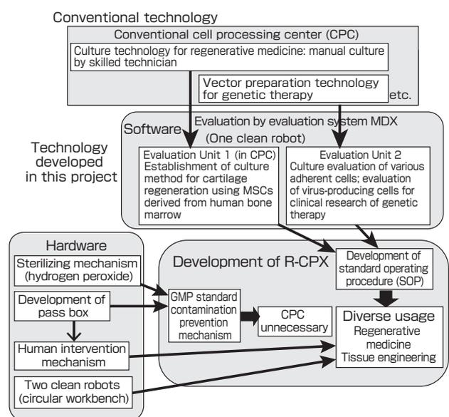
Fig. 1B Technological items in this project and the configuration diagram
