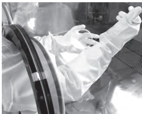
Fig. 5 Gloves that can be treated by hydrogen peroxide steam sterilization
