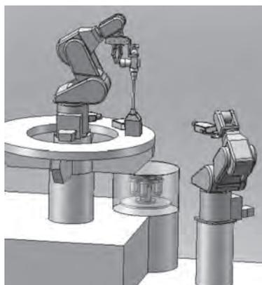
Fig. 4 Arrangement of the robot and rotating workbench
