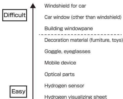
Fig. 6 Application of the switchable mirror thin film
