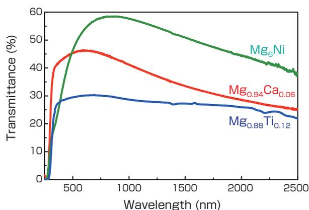
**Fig. 2 Comparison of the transmission spectra in the transparent state of the magnesium-nickel (Mg<sub>6</sub>Ni) switchable mirror, magnesium-titanium (Mg<sub>0.88</sub>Ti<sub>0.12</sub>) switchable mirror, and magnesium-calcium (Mg<sub>0.94</sub>Ca<sub>0.06</sub>) switchable mirror**
