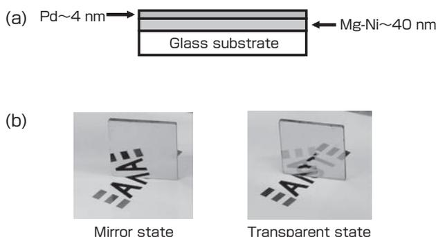
**Fig. 1 (a) Basic structure of the switchable mirror, and (b) the magnesium-nickel (Pd/Mg<sub>6</sub>Ni) switchable mirror thin film with excellent optical property developed at AIST**
