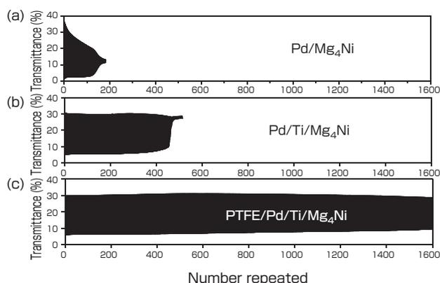
**Fig. 3 Comparison of switching durability**
