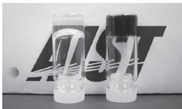
**Fig. 4 Photograph of hydrogel in inverted sample bottle (concentration at 1 wt%)**
