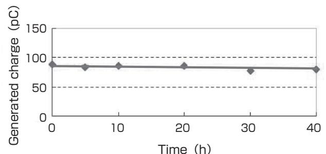
Fig. 10 Dependence of AlN sensor output on engine run time
