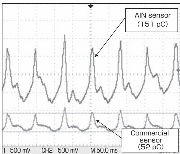
**Fig. 15 Response waveform of AlN sensor in four-cycle engine**
