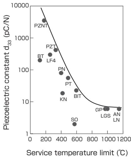
**Fig. 1 Relationship between piezoelectric constant  $d_{33}$  and service temperature limit**
