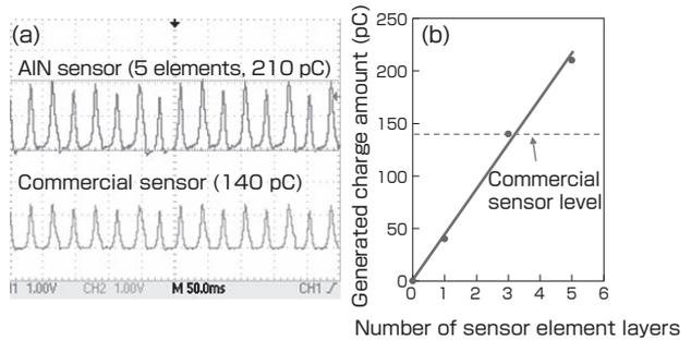
**Fig. 13** (a) Response waveform of AlN sensor, and (b) dependence of generated charge amount on number of sensor elements
