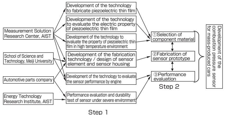
**Fig. 2 Elemental technologies for development of combustion pressure sensors for mass-produced cars and scenario for integration**
