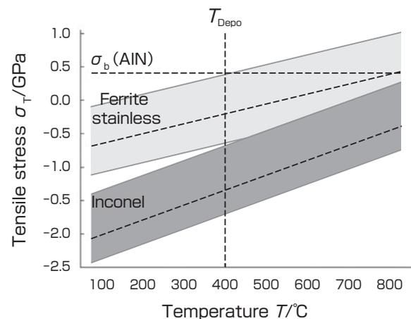
**Fig. 5** Temperature dependence of internal stress of AlN thin film formed on various substrate materials
