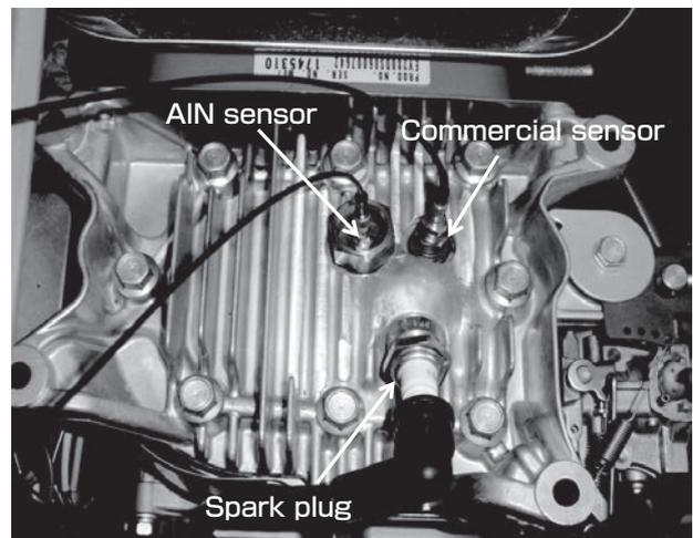
**Fig. 14** Appearance of four-cycle engine with sensors attached
