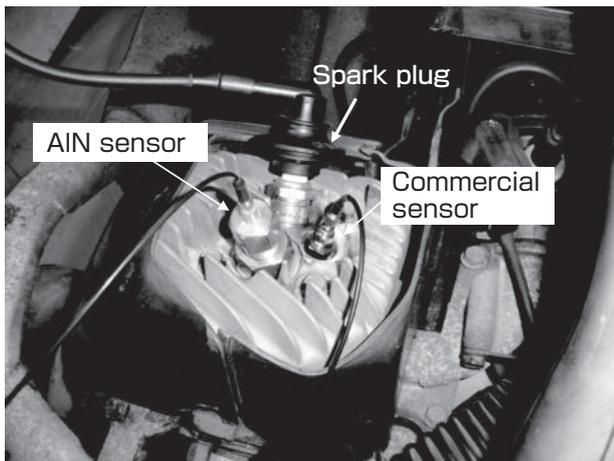
Fig. 8 Attachment of sensor to two-cycle engine
