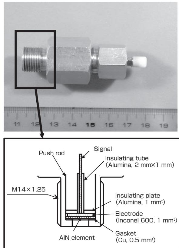
**Fig. 7 Appearance of AlN sensor and schematic diagram of interior structure**
