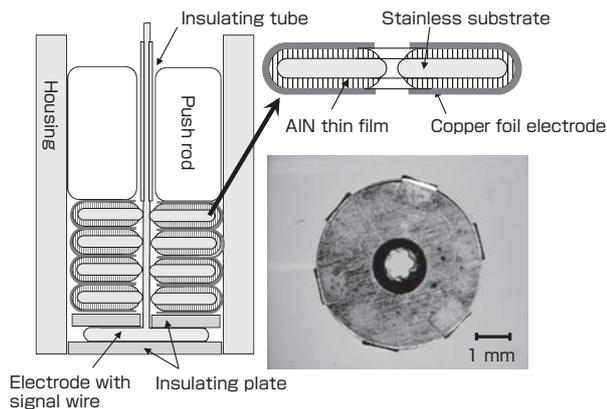
**Fig. 11** Diagram and photograph of laminated structure of AlN thin film sensor element
