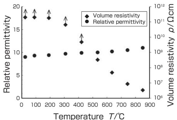
**Fig. 3** Temperature dependence of the relative permittivity and volume resistivity of AlN thin film
