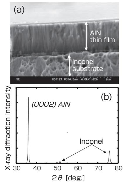
**Fig. 4** (a) Cross sectional SEM photograph and (b) XRD pattern of AlN thin film fabricated on Inconel substrate
