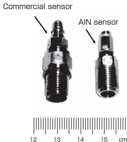
**Fig. 12** Appearance of fabricated AlN sensor prototype
