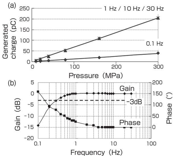
**Fig. 6 (a) Pressure dependence of generated charge of AlN element for frequency between 0.1~30 Hz, and (b) frequency response of gain and phase of AlN element against pressure change of 150 MPa**
