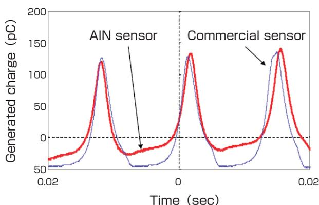
Fig. 9 Output waveform of sensor during operation of two-stroke engine
