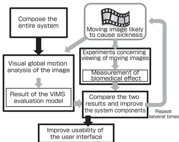
**Fig. 3 R&D procedure for the VIMS evaluation system**
