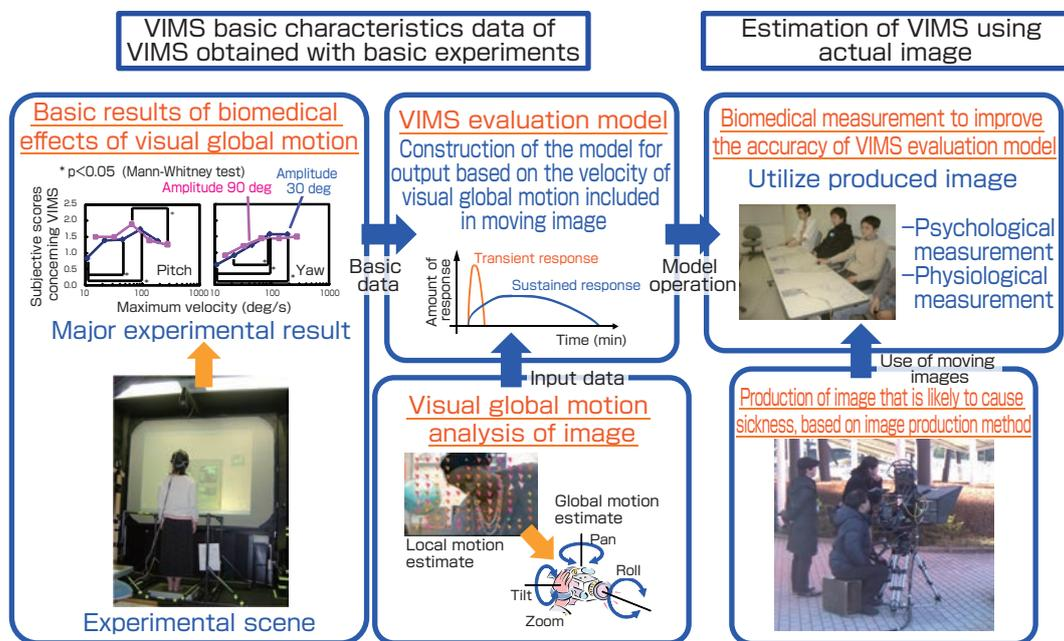
Fig. 4 Relationship of the elemental technology in the VIMS evaluation system
