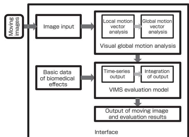
Fig. 2 Configuration of the VIMS evaluation system
