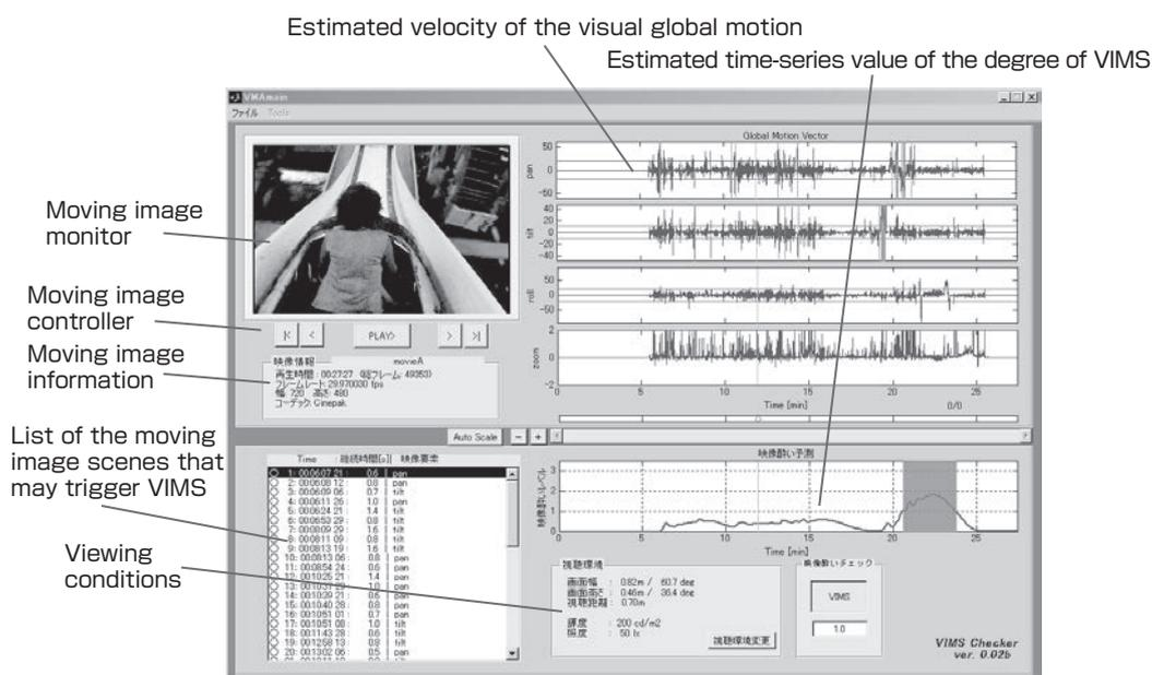
Fig. 6 Control window of the VIMS evaluation system
