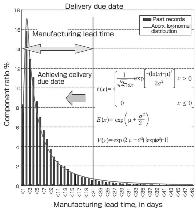
**Fig. 4 Distribution of manufacturing lead time**
