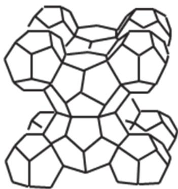
**Fig. 1 Crystalline structure of methane hydrate**
