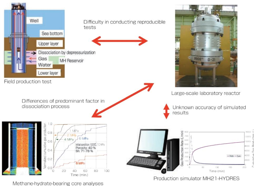
**Fig. 3 Large-scale laboratory reactor for resolving disadvantages of production tests, core analyses and production simulations** These issues are the main research concepts for establishing gas production methods and evaluating conditions in methane-hydrate-bearing layers.
