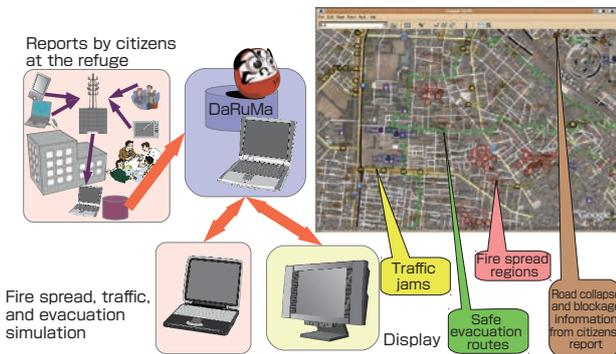
Fig. 8 System configuration for Toyohashi City demonstration experiment
