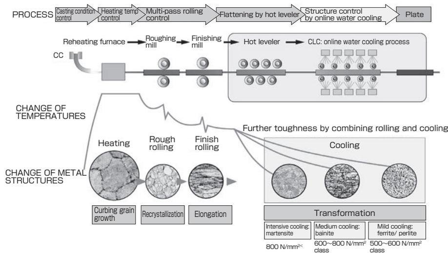
**Fig. 3 Microstructure control of steel plates and TMCP technology<sup>[3]</sup>**
