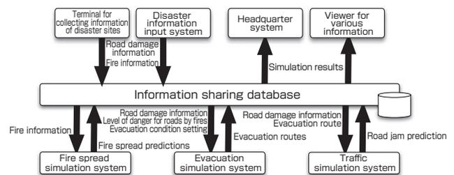
Fig. 9 System configuration for Toyohashi City demonstration experiment
