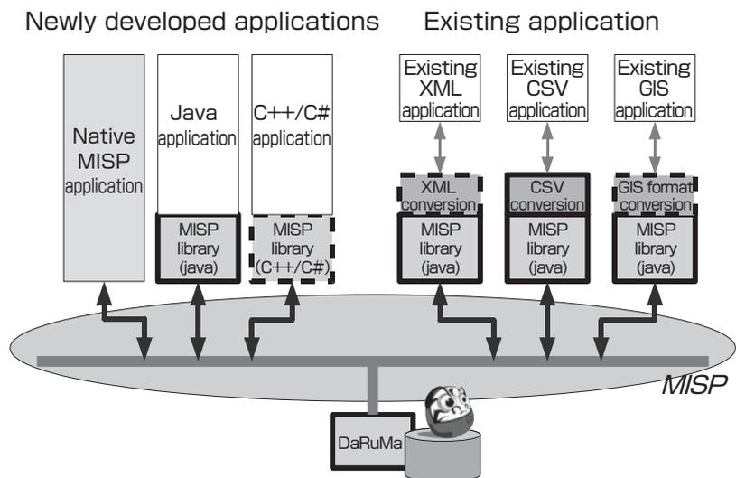
Fig. 6 System linkage by mitigation information sharing protocol (MISP) and DaRuMa
