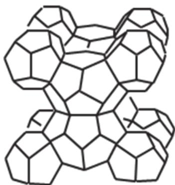
**Fig. 1 Crystalline structure of methane hydrate**
