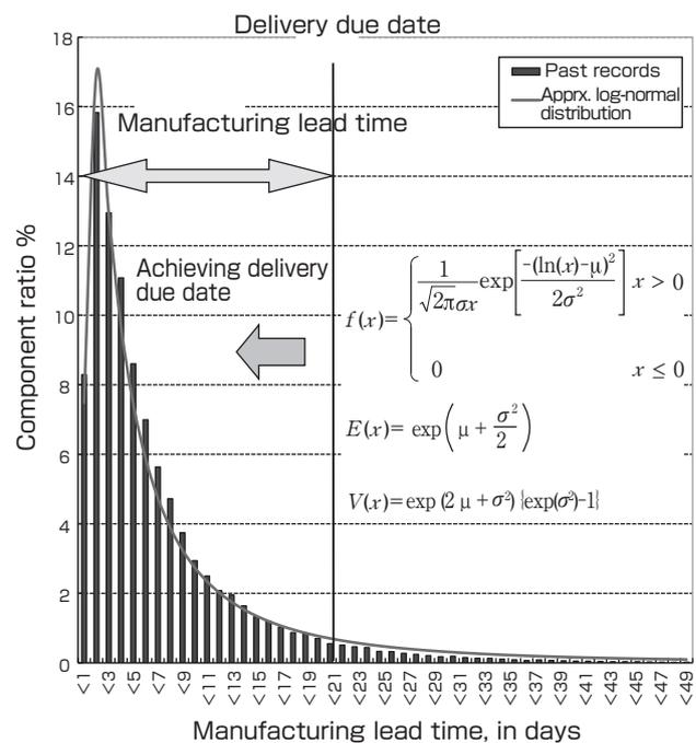
**Fig. 4 Distribution of manufacturing lead time**
