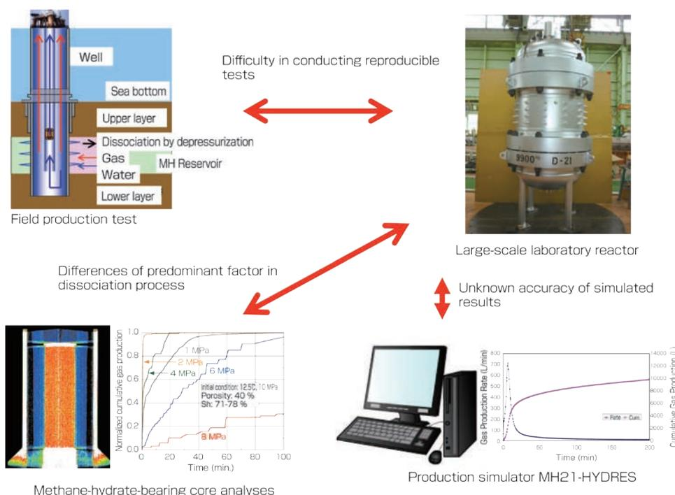
**Fig. 3 Large-scale laboratory reactor for resolving disadvantages of production tests, core analyses and production simulations**
