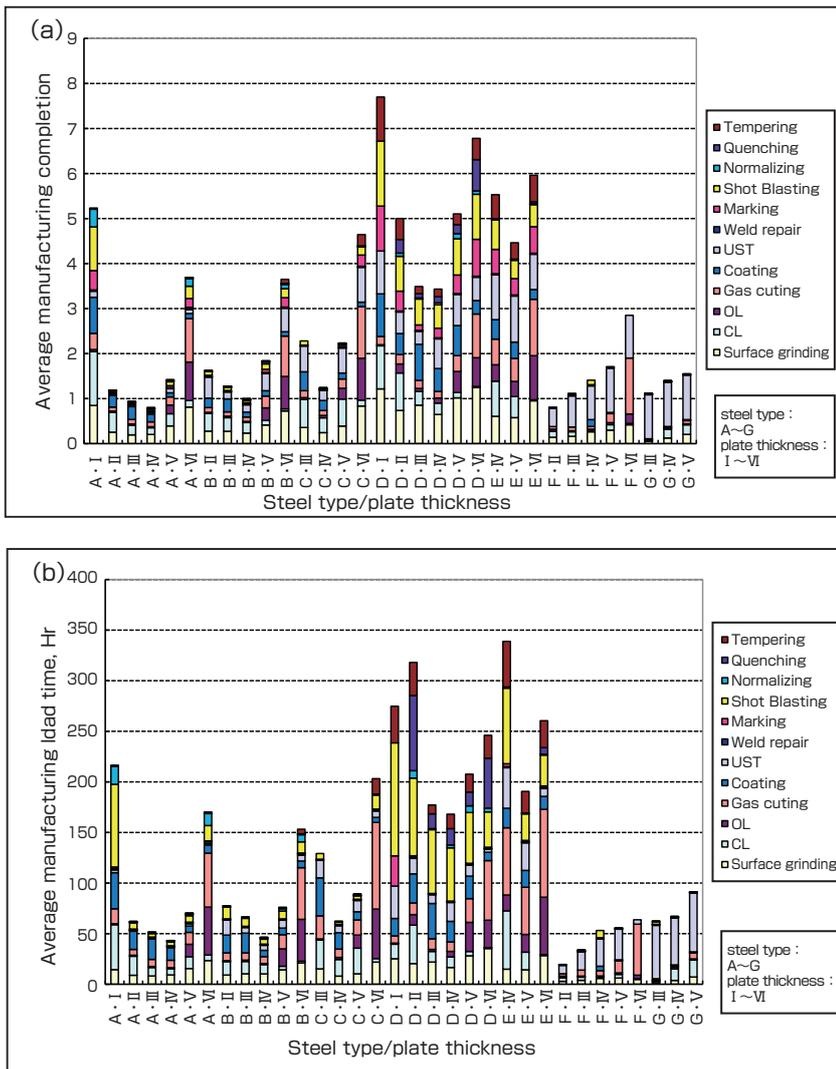
**Fig. 5 Average number of processes to be passed and the manufacturing lead time for individual product types**
