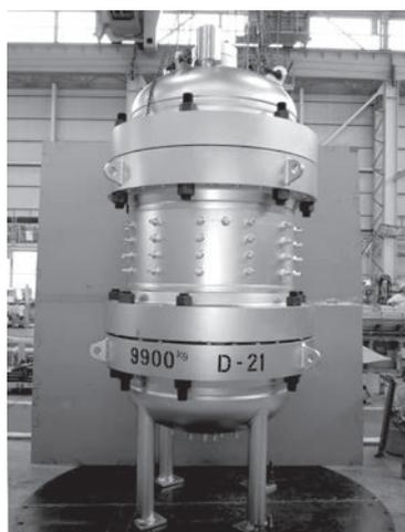
(a) High-pressure vessel of the large-scale laboratory reactor
