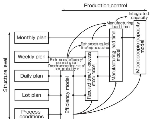
**Fig. 6 Production control multi-scale hierarchically structured model**
