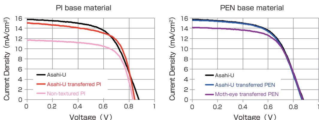
**Fig. 7 Current-density – voltage characteristics of the amorphous silicon solar cells fabricated on PI and PEN films**
