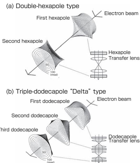
**Fig. 4 Construction and calculated electron-beam trajectories of spherical aberration correctors**
