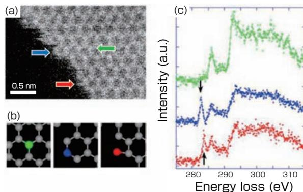
**Fig. 12 Observation of electronic states with low-voltage STEM-EELS**
