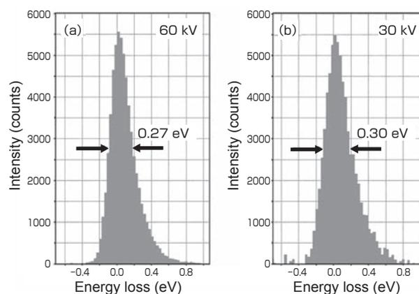
**Fig. 3 Evaluation of energy spread of low-voltage electron gun**
