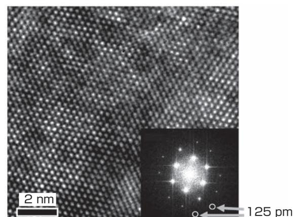
**Fig. 10 Performance examination of the second low-voltage microscope (TEM)**
