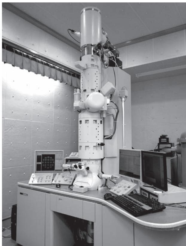
**Fig. 6** External view of the first experimental microscope (spherical aberration-corrected low-voltage TEM/STEM)
