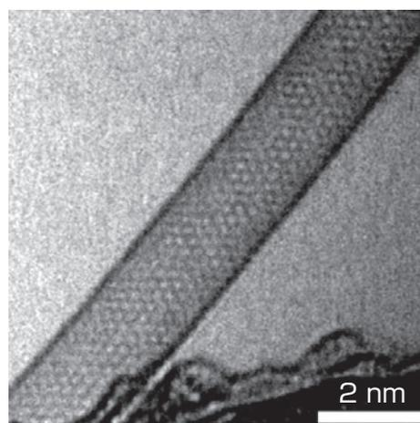
**Fig. 9 TEM image of a SWCNT recorded at an acceleration voltage of 30 kV**
