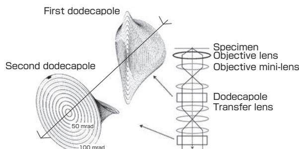
**Fig. 5 Construction and calculated electron-beam trajectory of new chromatic aberration corrector**
