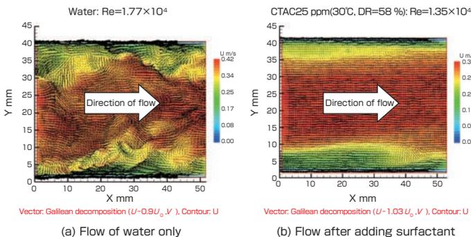
**Fig. 2 Changes in flow due to micelle network**
