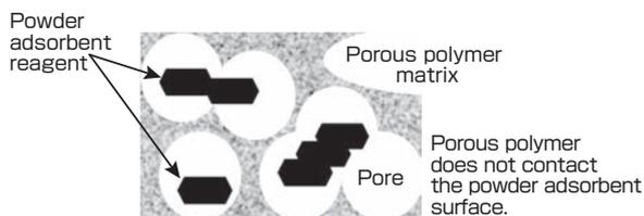
**Fig. 5 Schematic diagram of contactless supporting and shaping**
