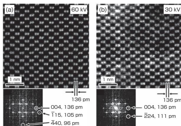
**Fig. 7** Performance examination of the first low-voltage microscope in STEM mode
