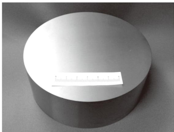
**Fig. 2 Photograph of a large-size WC-FeAl sintered body**
