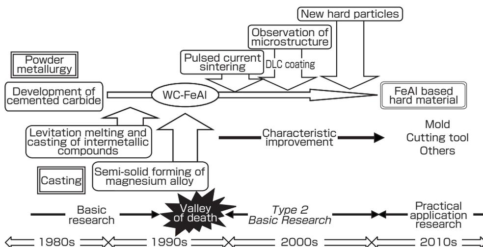
Fig. 7 Development process of WC-FeAl hard material
