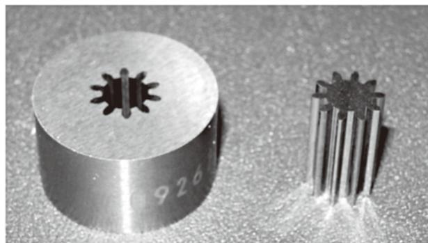
**Fig. 3 Photograph of the mold made using WC-FeAl**
