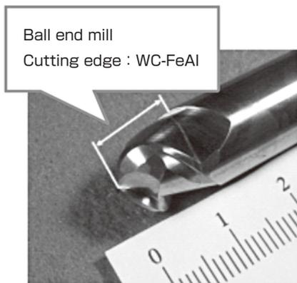
**Fig. 5 Prototype ball end mill made using WC-FeAl**
