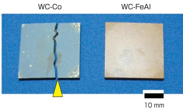
**Fig. 4 Photograph of WC-based hard materials quenched in water from 900 °C in the air**
