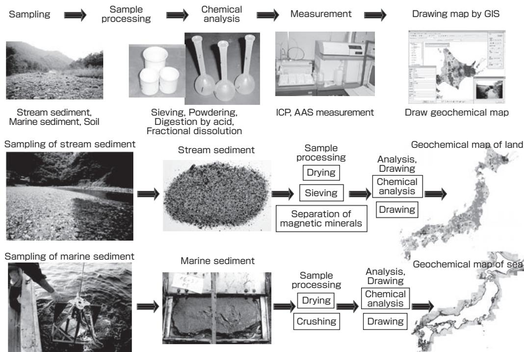
**Fig. 2 Scheme of making the geochemical map**
