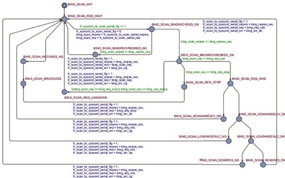
**Fig. 11 Cooperative behavior model for the measurement subsystem**
