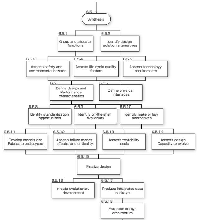
Fig. 4 Process of physical designing in IEEE 1220<sup>[11]</sup>
