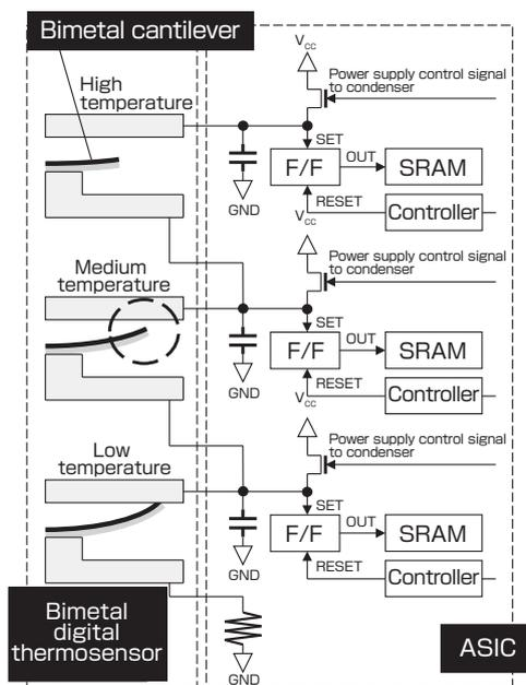
Fig. 4 Digital bimetal thermosensor
