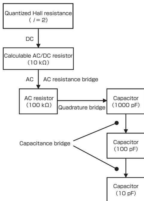
**Fig. 3 Capacitance standard based on quantized Hall resistance**
