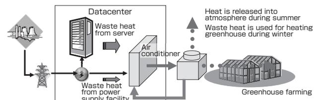
Fig. 6 Use of waste heat from datacenter in farming
