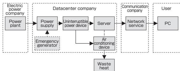
**Fig. 1 Energy flow of the datacenter**
