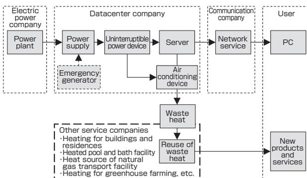
Fig. 5 Energy flow of the composite datacenter
