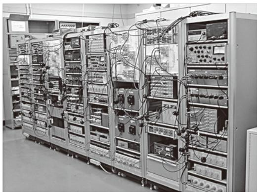
**Fig. 7 Capacitance standard based on quantized Hall resistance (national standard)**
