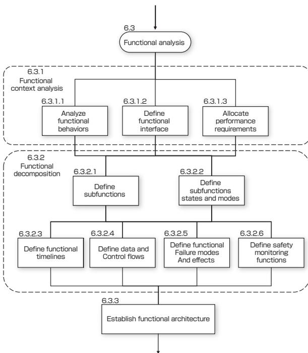
Fig. 3 Process of functional designing in IEEE 1220<sup>[11]</sup>
