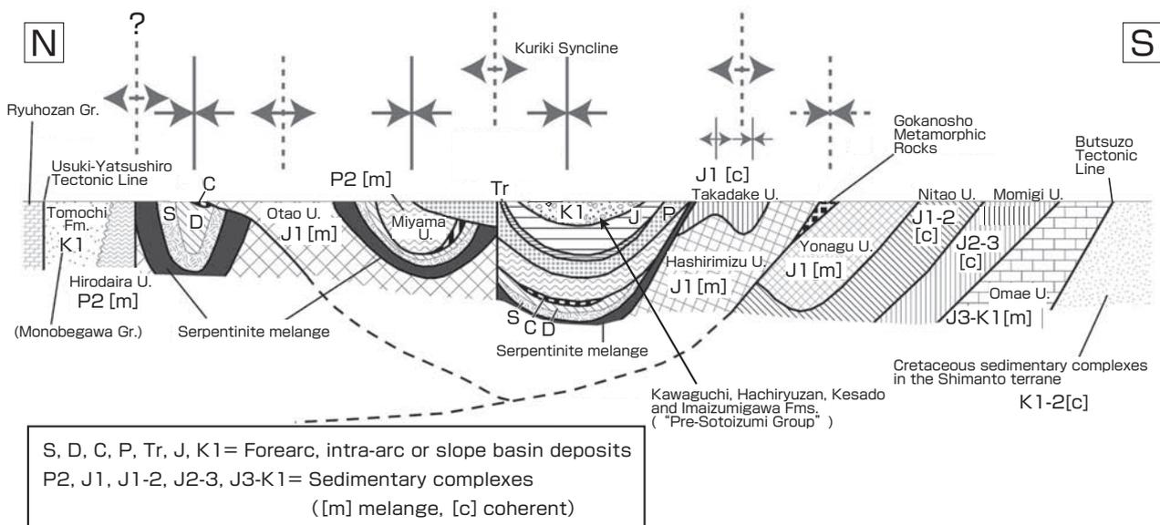
**Fig. 7 Schematic cross section for the south to central area of the GMJ Tomochi 1:50,000 sheet area.**
