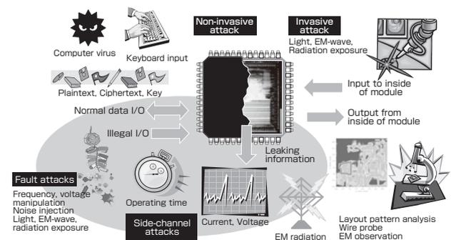
Fig. 2 Various physical attacks against cryptographic modules.
