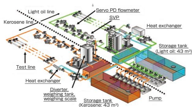
**Fig. 4 Diagram of the hydrocarbon high-flow calibration facility.**
