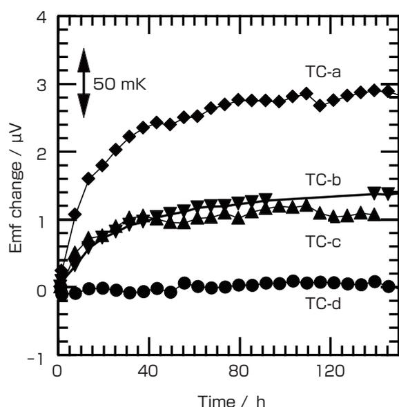
Fig. 13 Drift of the Pt/Pd thermocouples using palladium wires from different lots.
