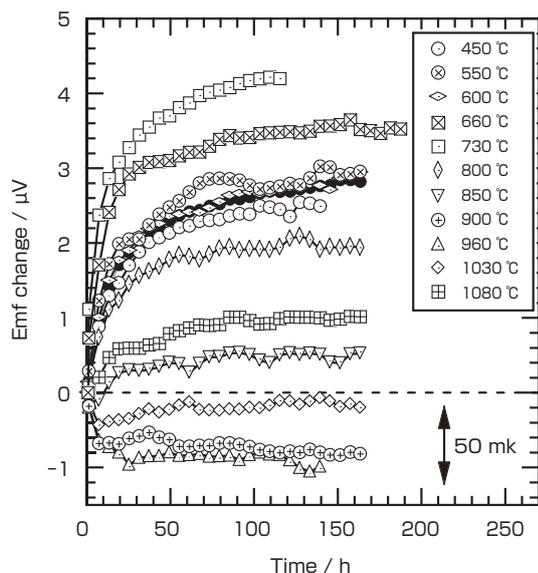
**Fig. 15** Drift of the Pt/Pd thermocouples annealed at different temperatures as final heat treatment.
