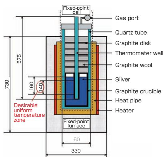
Fig. 3 Schematic diagram of the Ag fixed-point device.
