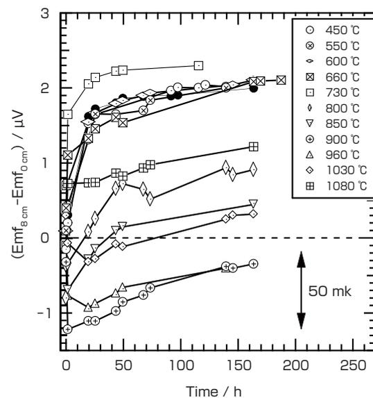
**Fig. 16** Inhomogeneity of the Pt/Pd thermocouples annealed at different temperatures as final heat treatment.
