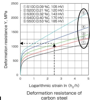
$$\text{Processing pressure} = \text{Restraint coefficient} \times \text{Deformation resistance}$$
