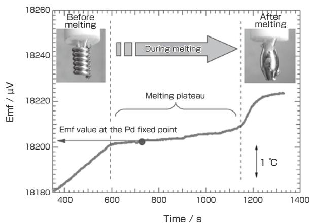
Fig. 8 Melting curve at the Pd fixed point.
