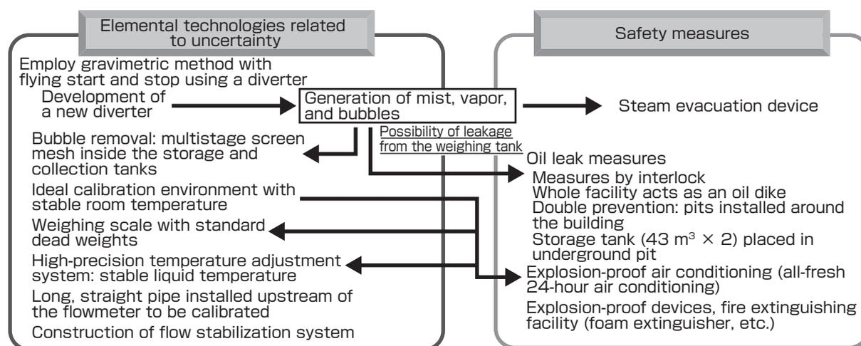
Fig. 3 Elemental technology developed for hydrocarbon high-flow standard.
