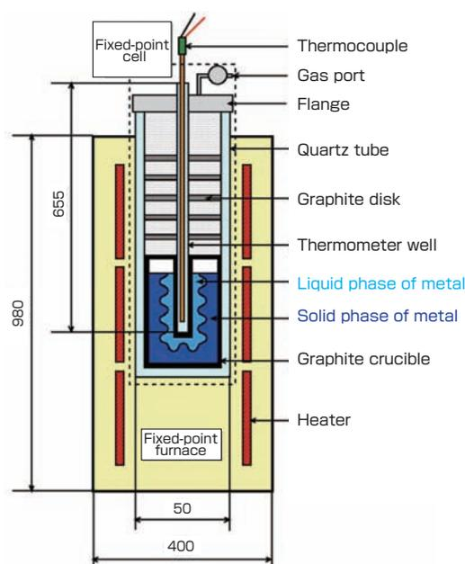
Fig. 4 Schematic diagram of the Cu fixed-point device.
