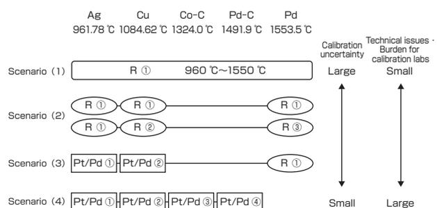
**Fig. 2 Comparison of the scenarios for thermocouple traceability.**
