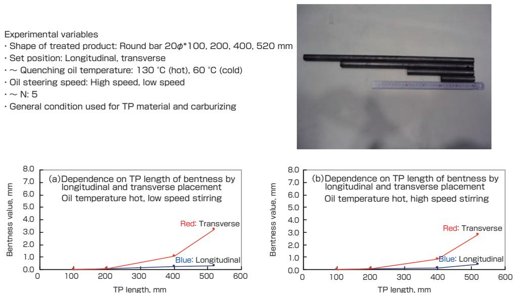
Fig. 5 Example of derivation of experimental formula in heat treatment.
