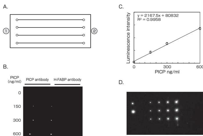
**Fig. 7** Schematic diagram of the microchip substrate with micro flow channel (A) and the PICIP detection image using this chip (B), calibration curve (C) and the image of chemiluminescence when antibody of arbitrary amount is fixed on each flow channel (D).
