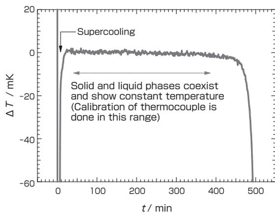
Fig. 5 Freezing curve at the Cu fixed point.
