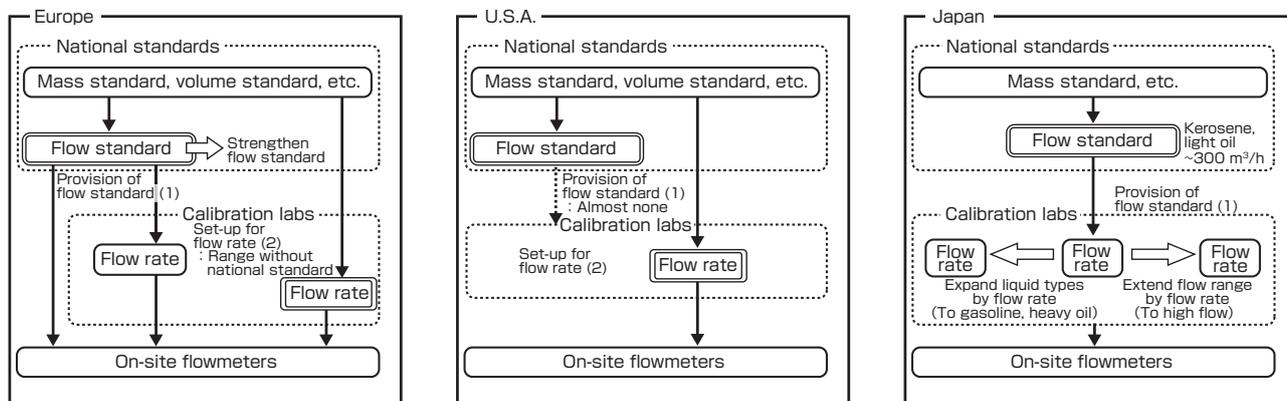
Fig. 1 Outline of the hydrocarbon flow standard system.
