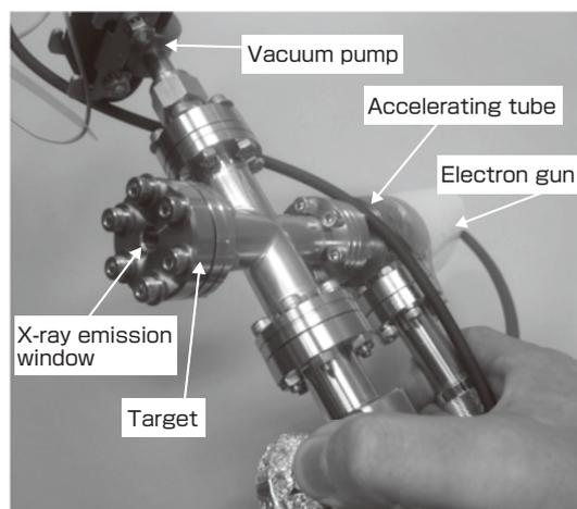
Fig. 7 Main body of the X-band ultra-small electron accelerator.
