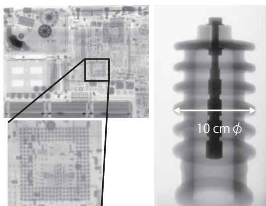
**Fig. 4 X-ray transmission image with input power 20 J.**
