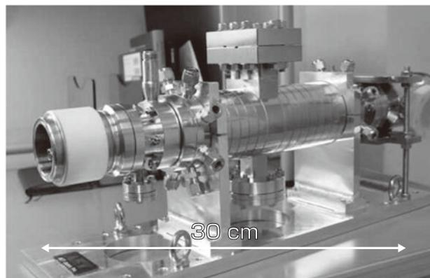
**Fig. 6** First part of C-band electron accelerator.
