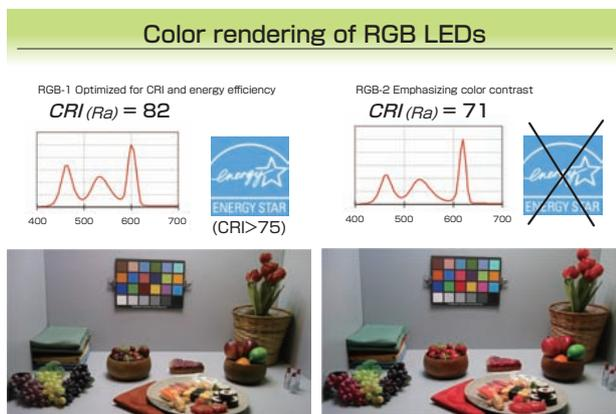
Fig. 2 Color rendering of RGB LEDs.
