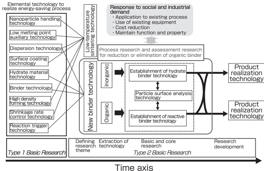
Fig. 7 Building of low-environment load process and mutual relationship in existing ceramic manufacturing steps.
