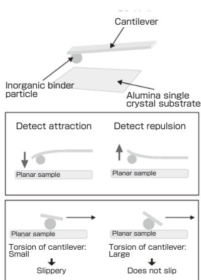
**Fig. 6 Measurement of inter-surface interactive force.**
