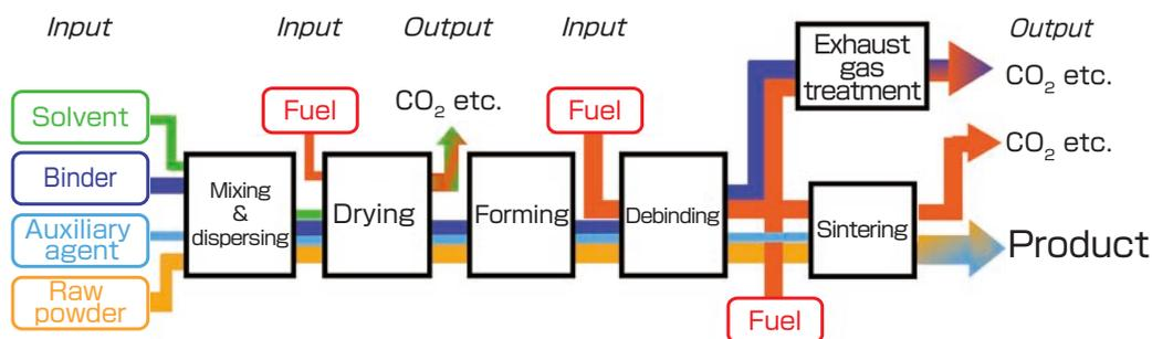
Fig. 1 Steps of ceramic manufacturing and the flow of resource materials.
