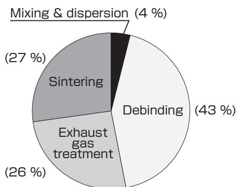
**Fig. 2 Percentage of consumption energy in each process (all are laboratory level; energy required for powder production is not included).**
