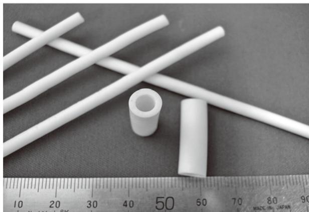
**Fig. 5 Alumina ceramics fabricated using inorganic binder technology.**
