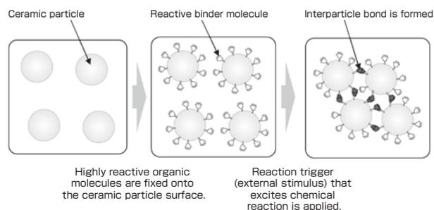
Fig. 4 Fixing of organic molecule and application of reaction trigger to reduce the amount of organic binder.
