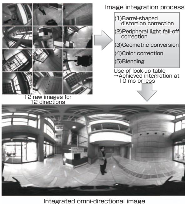
**Fig. 4 High quality and high speed image integration.**
