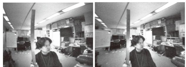
**Fig. 5 Lens distortion correction.** The person in the photo is holding a ruler in his hand. In the left photo, the ruler is arched since this is the image before correction. On the right is the corrected image. The distortions of the line of the ceiling and other parts are also corrected.
