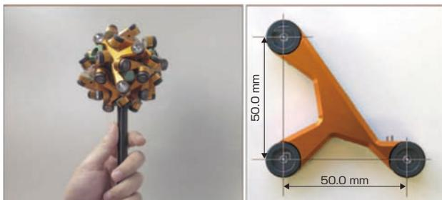
**Fig. 3 Stereo omni-directional system.** The left photo shows the camerahead (diameter of 116 mm). Right photo is the stereo camera unit. The three cameras are arranged at right angles to each other in a single plane.
