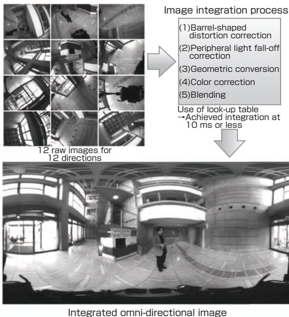
**Fig. 4 High quality and high speed image integration.** The omni-directional image is produced in high quality and in high speed from 12 raw images that include lens distortion and peripheral light fall-off. Although it is difficult to present the omni-directional image in 2D, we present the image in Mercator projection, as in a world map.
