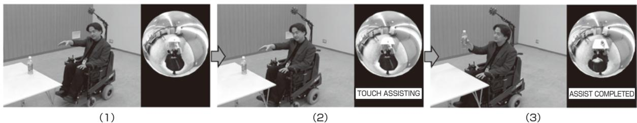
**Fig. 17** Automatic assistance is provided to the position that allows the hand to reach the bottle, by recognizing the rider’s gesture.
