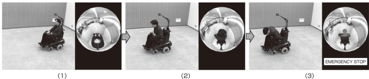
**Fig. 16** Emergency stop when an abnormality in the rider’s seating position is detected.
