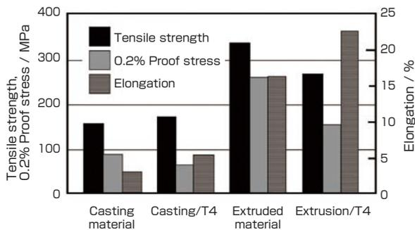
**Fig. 6 Mechanical property of noncombustible magnesium alloy (AMX602).**
