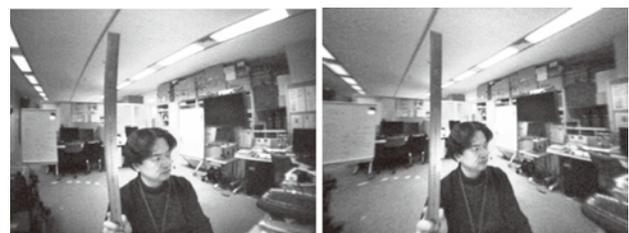
**Fig. 5 Lens distortion correction.**
