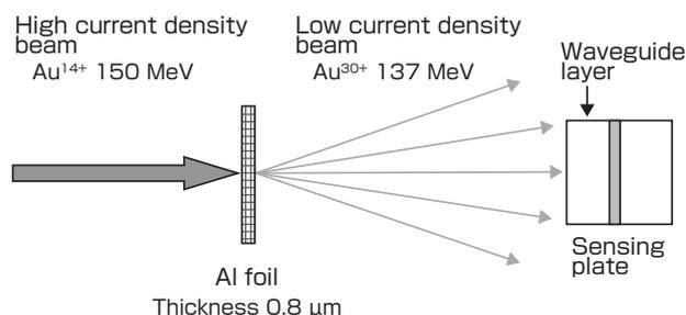
Fig. 5 Ion irradiation method used in nanopore formation.
