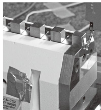
**Fig. 5 Exterior view of step gauge (measurement surface is arranged in comb-tooth form).**
