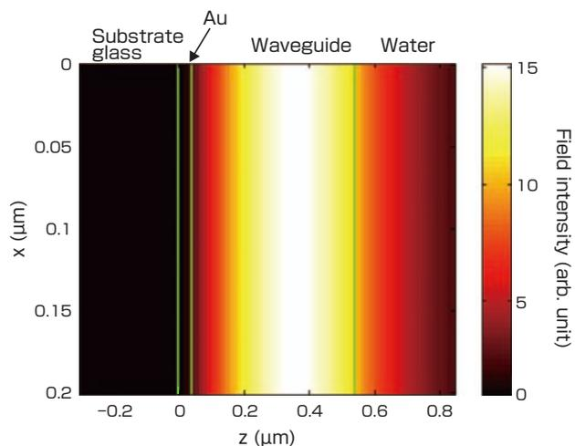
**Fig. 3 Simulation result of the electric field profile in a waveguide in which a waveguide mode is excited.**
