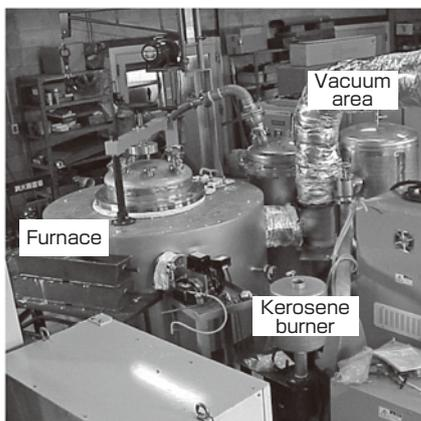
**Fig. 4 Smelting furnace for noncombustible magnesium alloy equipped with reduced pressure refinement mechanism (capacity 100 kg).**
