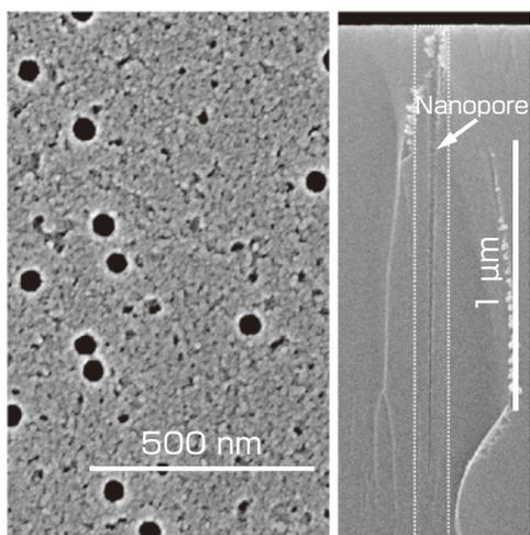
Fig. 6 SEM photographs of the surface (left) and cross section (right) of nanopores formed on a thermally-grown  $\text{SiO}_2$  film.
