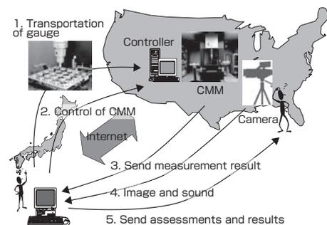
Fig. 13 Remote calibration technology for CMM.
