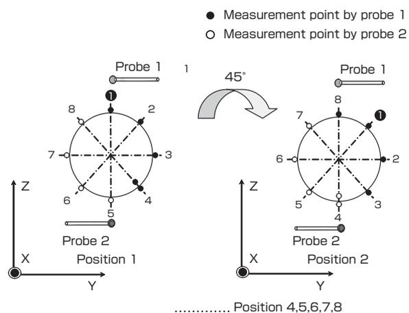
Fig. 15 Multiple measurement method of cylinder.
