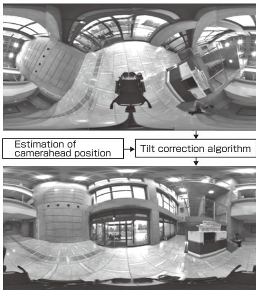
**Fig. 6 Estimation of camerahead position and tilt correction.**
