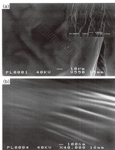
**Fig. 3** Surface structure of oxide film in Mg-5Ca binary alloy.
