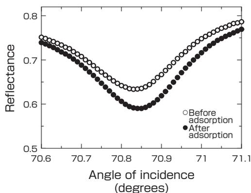
**Fig.15** Reflectance property before and after adsorption of streptavidin with gold nanoparticles (immunogold conjugate, concentration 10 pM) on biotin, observed using optical absorption detecting monolithic sensing plate.
