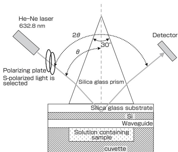
**Fig.12** Optical setup used in molecular detection using the monolithic sensing plate.
