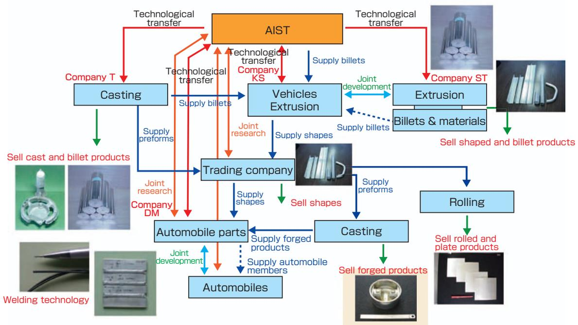
Fig. 9 Mass production system for noncombustible magnesium alloy.
