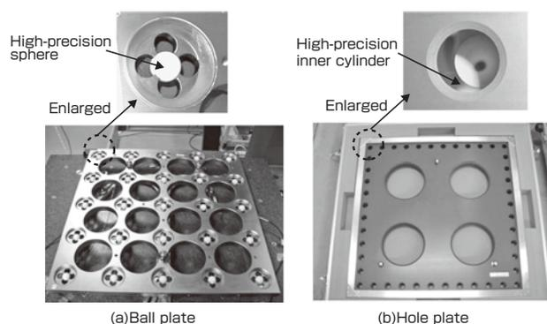
Fig. 7 Two-dimensional standard.
