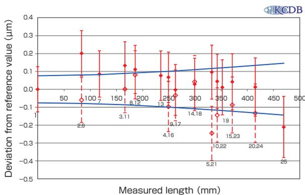
**Fig. 10 Result of international comparison for ball plate (CCL-K6).**
