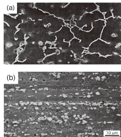
**Fig. 5 Structure of noncombustible magnesium alloy (AMX602).**
