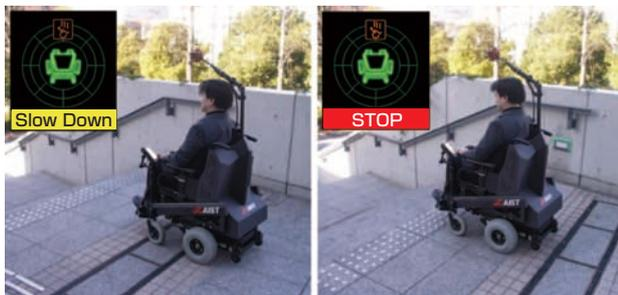
**Fig. 15 Detection of descending stairs.**
