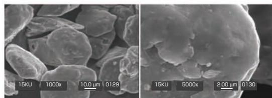
**Fig. 8 Crushed particles of noncombustible magnesium alloy (AMX602) (sieve gauge 38  $\mu\text{m}$ ).**
