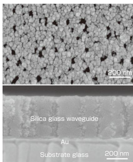
Fig. 7 SEM photographs of the surface (top) and cross section (bottom) of the sensing plate with nanopores.
