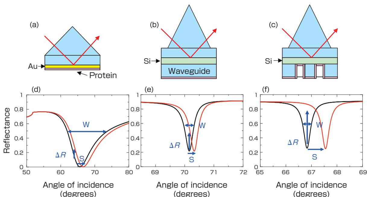
**Fig.14** Conceptual diagram of molecule adsorption in the SPR sensor (a), the EFC-WM sensor without nanopores (b), and the EFC-WM sensor with nanopores (c). (d), (e), and (f) show the calculation results of reflectance property before and after the molecule adsorption in (a), (b), and (c), respectively.
