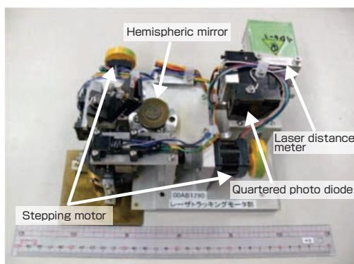
Fig. 14 Laser tracking interferometric distance meter.
