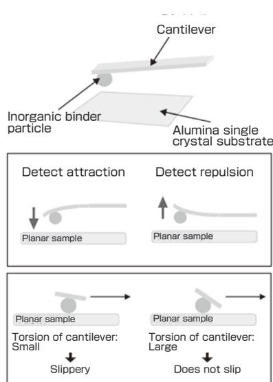
**Fig. 6 Measurement of inter-surface interactive force.**
