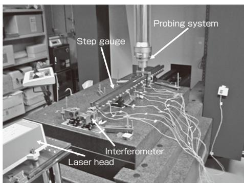
Fig. 6 Step gauge calibration system.
