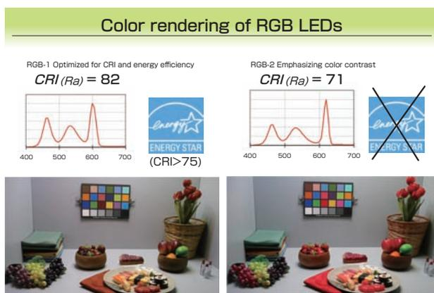
Fig. 2 Color rendering of RGB LEDs.
