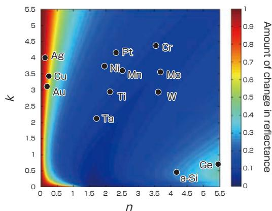
**Fig.10** Calculation result of relationship between the complex refractive index of the reflective film material and detection sensitivity. The black dots in the graph show the complex refractive index of some materials that may be used as the reflective film.
