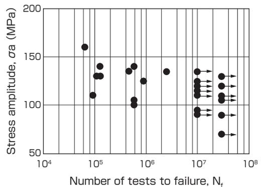
**Fig. 7 Endurance strength assessment of noncombustible magnesium alloy (AMX602).**
