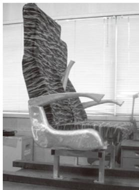
**Fig. 12 Railroad vehicle seat made of noncombustible magnesium alloy (AMX602).**
