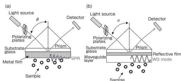
Fig. 2 (a) Optical configuration used in the SPR sensor. (b) Optical configuration used in the EFC-WM sensor.
