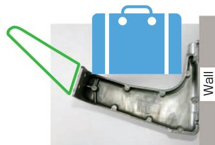
**Fig. 11 Luggage shelf support made of noncombustible magnesium alloy (AZX912).**
