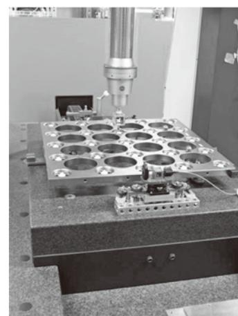
Fig. 8 Ball plate calibration.
