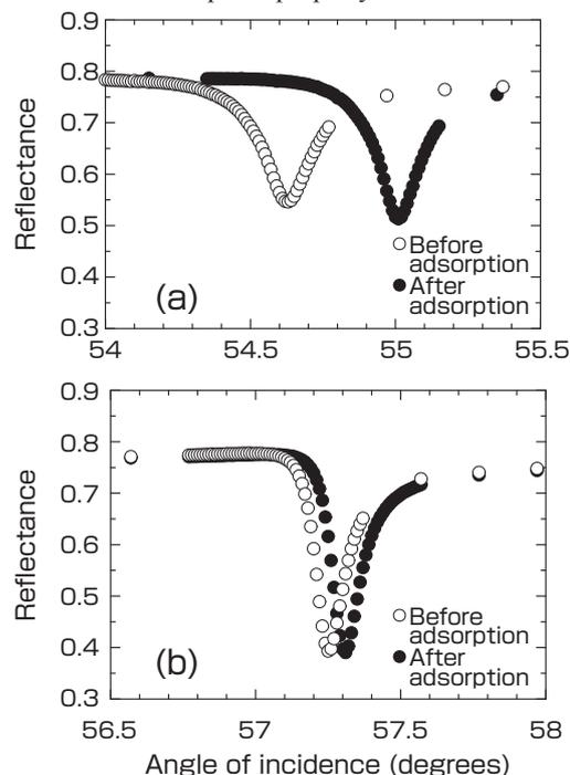
Fig. 8 Reflectance property before and after adsorption of streptavidin on biotin observed using the sensing plate with nanopores (a) and without nanopores (b).
