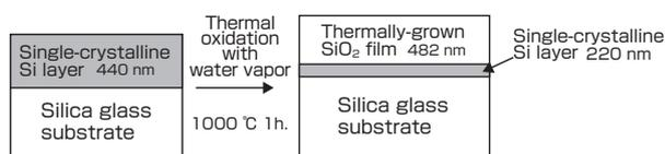
**Fig.11** Explanation of the process for fabricating the sensing plate by thermal oxidation of the single-crystalline Si layer of the SOQ substrate.
