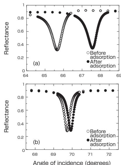
**Fig.13** Reflectance property before and after adsorption of streptavidin on biotin observed using the monolithic sensing plate with nanopores (a) and without nanopores (b). The concentration of streptavidin was 1.5 μM.
