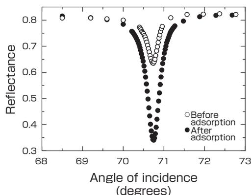
**Fig.16** Reflectance property before and after adsorption of streptavidin dyed with Coomassie Brilliant Blue G-250 (concentration 100 pM) on biotin, observed using optical absorption detecting monolithic sensing plate.
