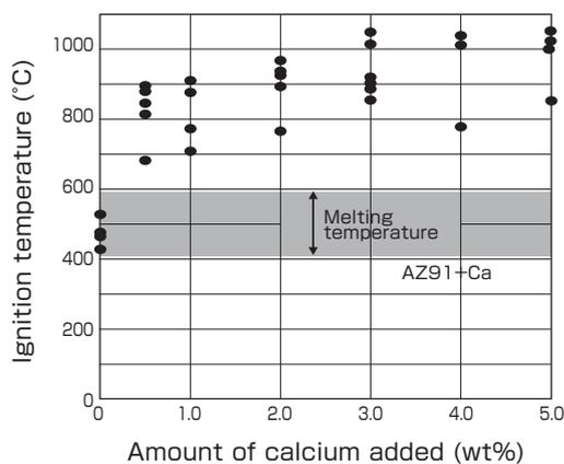
Fig. 1 Ignition temperature of noncombustible magnesium alloy (AZX912).
