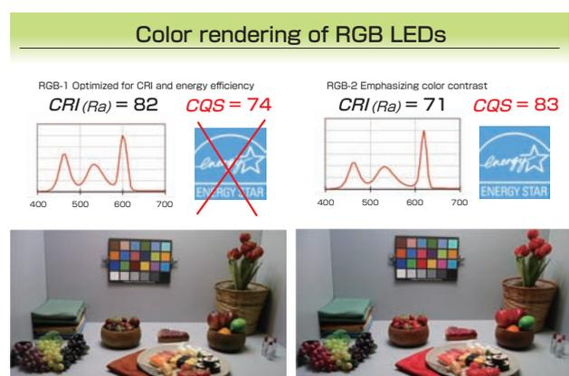
Fig. 3 Color rendering of RGB LEDs.
