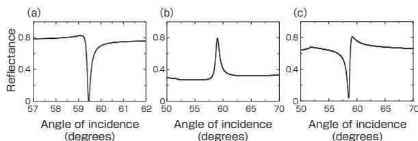
**Fig. 9** Calculation results of incident angle dependency of reflectance when Au (a), W (b), and Si (c) are used as reflective films. The thicknesses of reflective films are 40, 20, and 30 nm, respectively.
