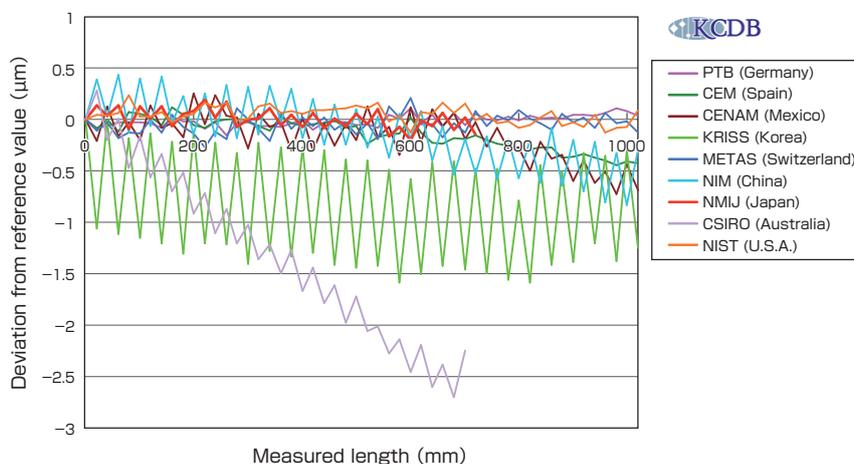
Fig. 9 Result of international comparison for step gauge (CCL-K5).
