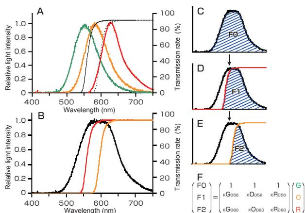
**Fig.3 Outline of technology for dividing and measuring three luminescence colors using two filters.**
