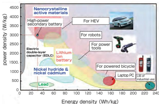
Fig. 1 Industrial products realized by innovations in battery technology.
