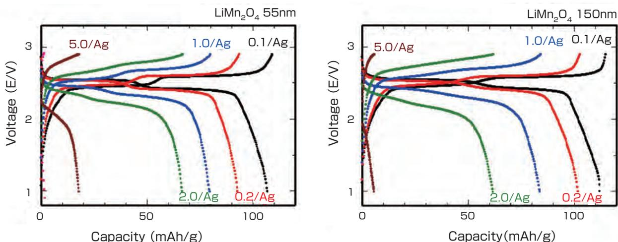
Fig. 10 Output property of lithium battery using nanocrystal electrode.
