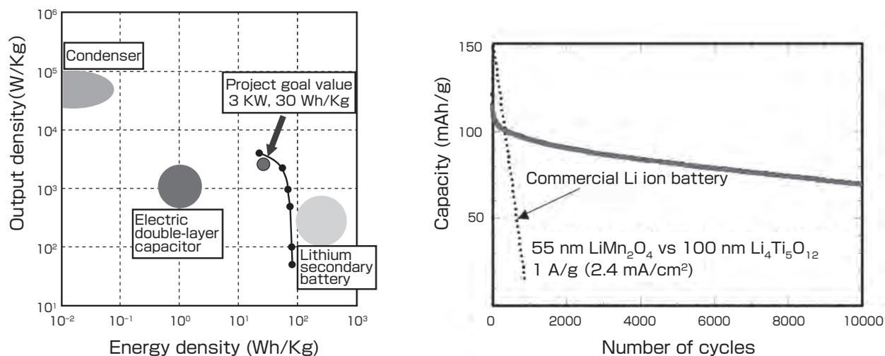
Fig. 11 Ragone plot of battery performance of prototype and charge-discharge cycle property (higher performances compared to existing batteries were observed for both items).
