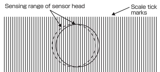
Fig. 13 Scale measurement size of rotary encoder.
