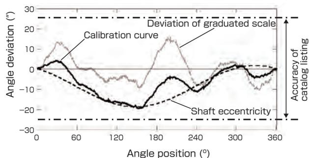
Fig. 3 Example of deviation factors in calibration curve.
