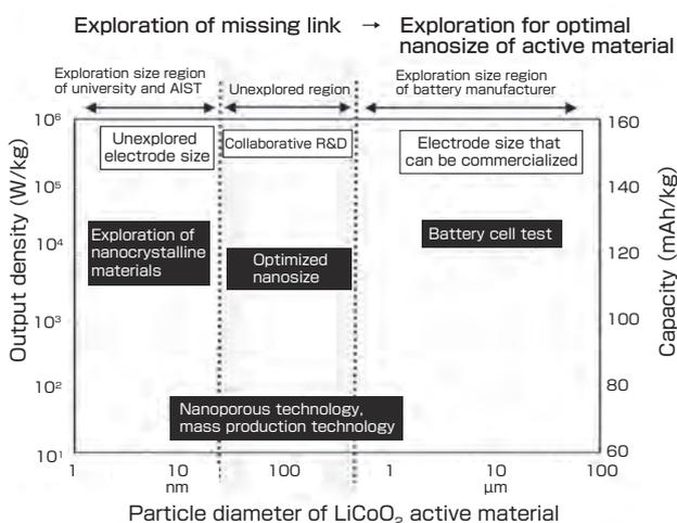
**Fig. 8 Exploring active material size in the missing region to optimize the electrode property.**
