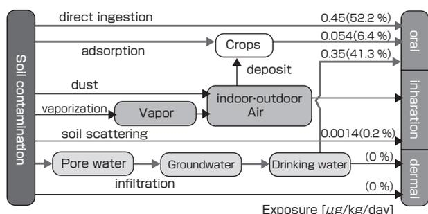
**Fig.6 The result of exposure rate and partition from contaminated soil by arsenic.**
