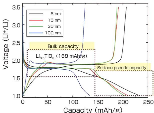
**Fig. 6 Charge-discharge curve of nanocrystalline titania.**
