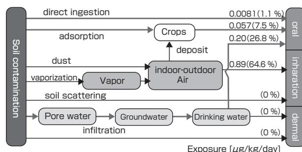
**Fig.7 The result of exposure rate and partition from contaminated soil by TCE.**
