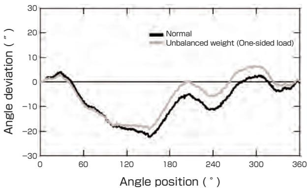
**Fig. 9 Change in calibration value of internal rotary encoder caused by load.**
