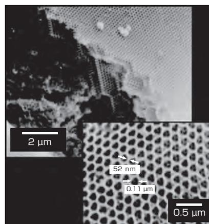
Fig. 5 Titania nanoporous electrode.
