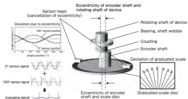
Fig.2 Concept of angle deviation factor of rotary encoder.
