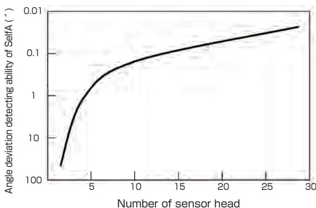
Fig. 12 Relationship between number of sensor head of SelfA and achieved accuracy.
