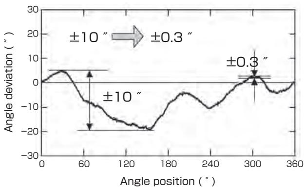
**Fig. 10 Calibration value of rotary table (static angle deviation).**
