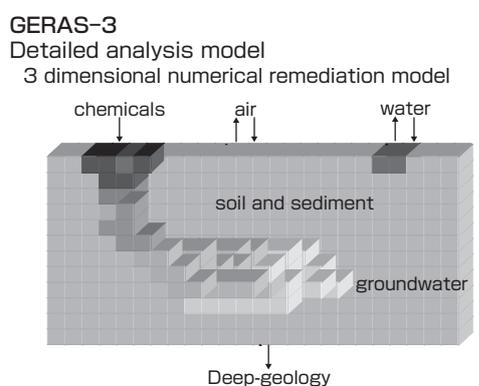
**Fig.4 Layered structure of geo-environmental risk assessment system GERAS.**
