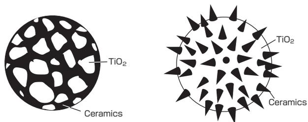
Fig. 2 Muskmelon-form and *kompeito*-form TiO<sub>2</sub> photocatalytic particles.
