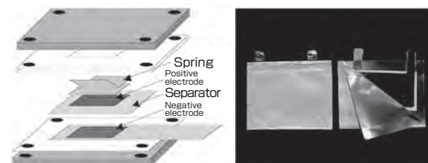
**Fig. 9 Structure and photograph of laminated battery cell prototype.**
