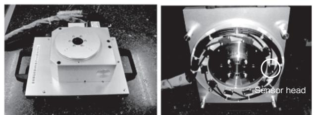
Fig. 8 Rotating table equipped with self-calibratable rotary encoder "SelfA".
