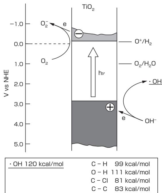
**Fig. 1 Energy level and photocatalysis of titanium dioxide.** V = electrical potential, NHE = normal hydrogen electrode. V vs. NHE is potential against normal hydrogen electrode, or potential when normal hydrogen electrode is used as standard.  $h\nu$  = energy of light.
