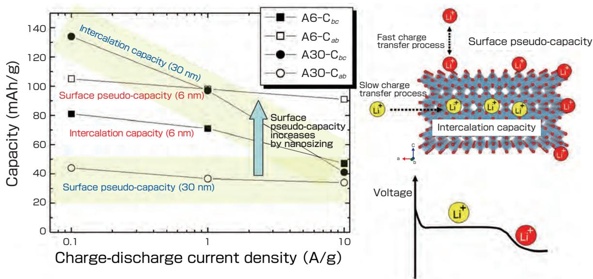
Fig. 7 Pseudo-capacity mechanism of nanocrystalline titania surface and its high-rate charge-discharge property.
