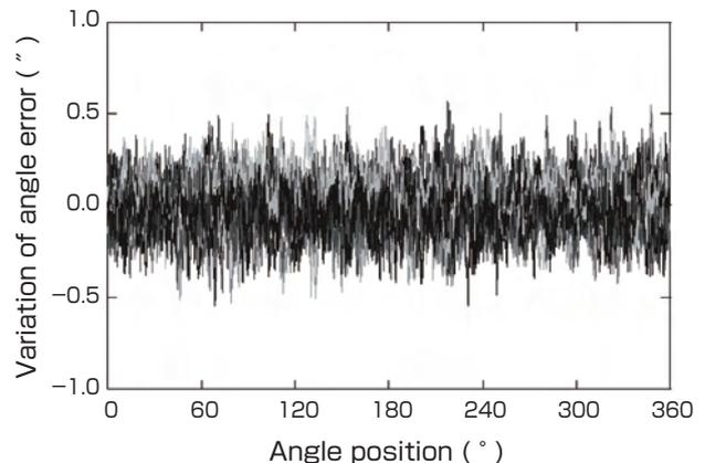
**Fig. 11 Reproducibility of calibration value of rotating table (dynamic angle deviation).**
