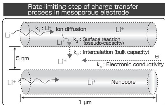
Fig. 3 Charge transfer process and rate-controlling step within electrode.
