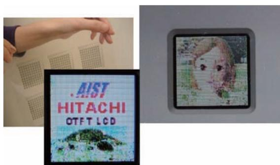
Fig. 6 Development of organic TFT driven color LC display.
