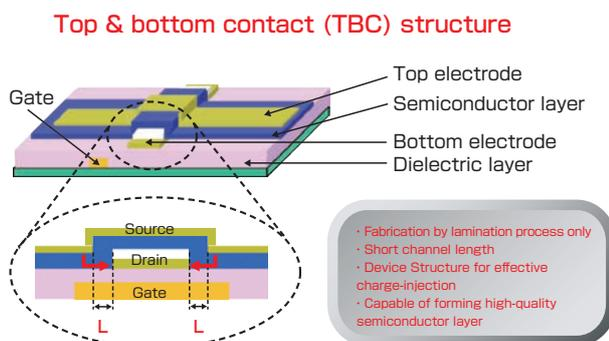
**Fig. 4** Top & bottom contact (TBC) structure for forming all-printed element.
