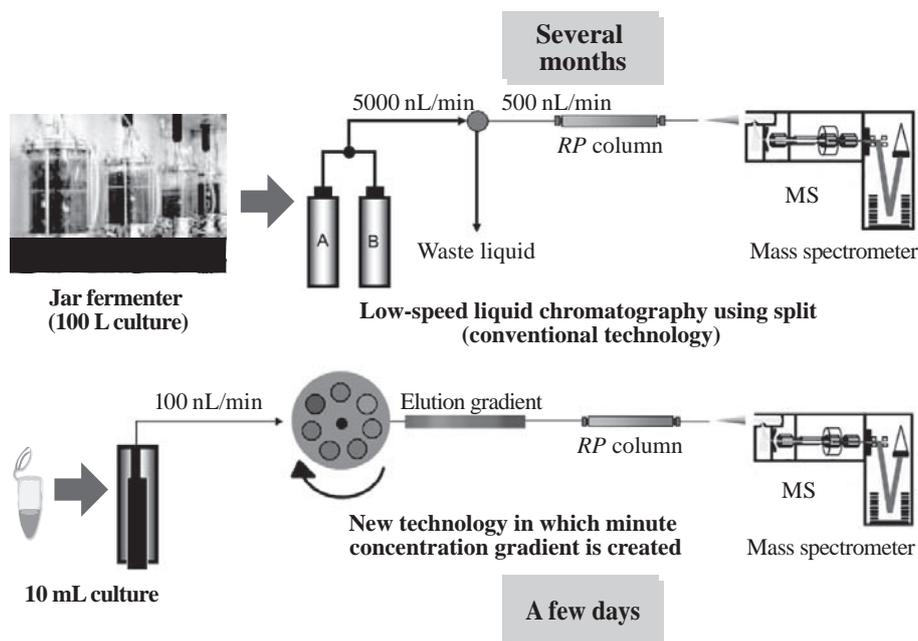
**Fig. 2 Comparison of new and conventional technologies.**
