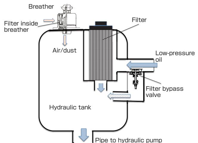
**Fig. 7 Schematic diagram of hydraulic tank and filter/breather**
