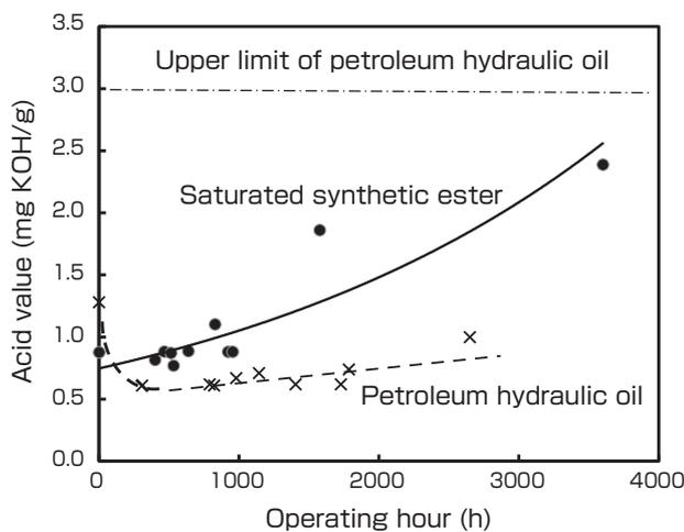
**Fig. 12 Acid value change of bio-oil of saturated fatty acid synthetic ester base oil<sup>[48]</sup> and that of petroleum hydraulic oil during field test of construction machinery,**
