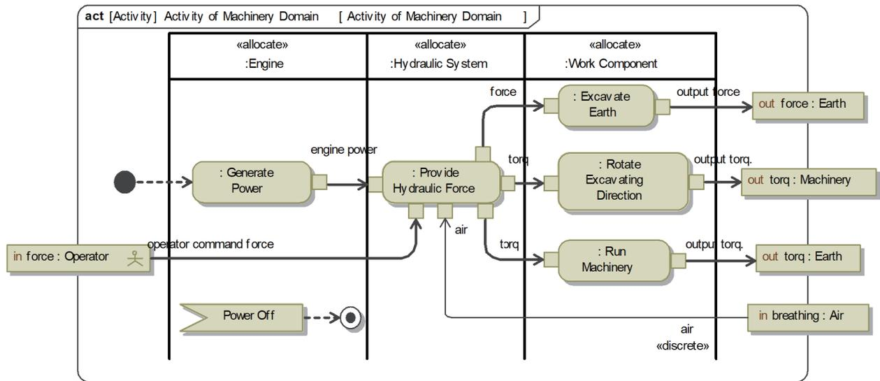
Fig. 5 Activity diagram of construction machinery domain
