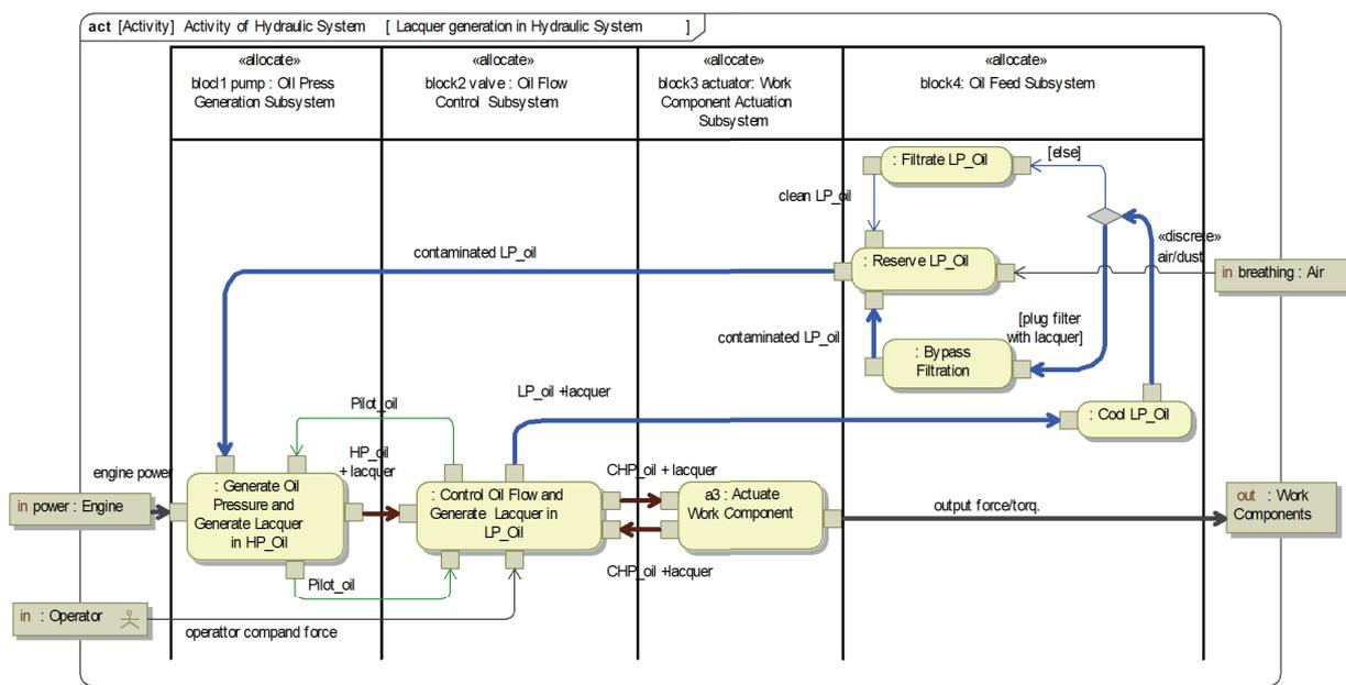
**Fig. 9 Activity diagram for lacquer formation and its behavior of bio-oil in hydraulic system**
