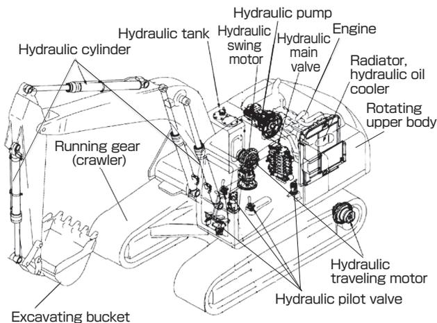
**Fig. 1 Exterior of construction machinery and arrangement of hydraulic devices<sup>[1]</sup>**
