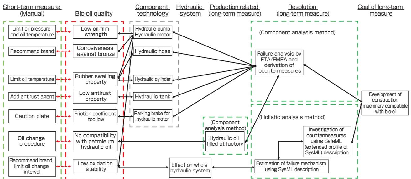
**Fig. 3 Scenario for development of construction machinery compatible with bio-oil**
