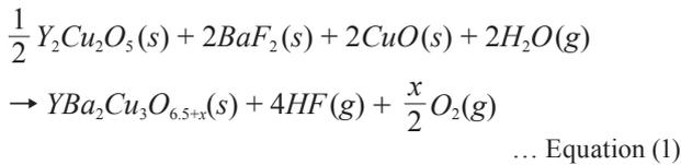
In this reaction, HF gas is generated as a reaction product (Fig. 7). This conversion reaction enables epitaxial growth. We first analyzed the reaction mechanism, and found that the growth rate is determined by the exhaust speed of HF gas ( $V_g$ ) and steam partial pressure ( $P_{H_2O}$ ) and total pressure ( $P_t$ ) and others.<sup>[20]</sup>
