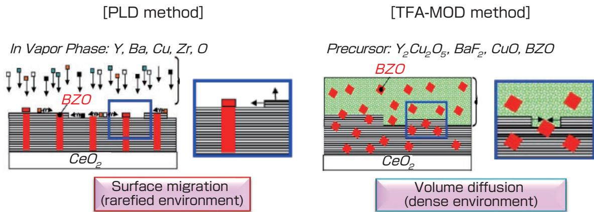
Fig. 12 Different growth mechanisms for films containing artificial pinning centers in PLD and TFA-MOD methods
