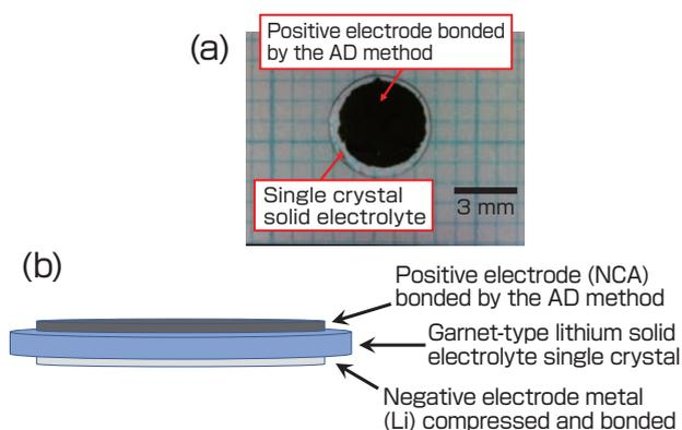
**Fig. 12 (a) NCA electrode film formed on garnet-type lithium solid electrolyte single crystal substrate using the AD method; (b) schematic diagram of developed all-solid-state lithium secondary battery**
