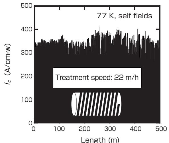
Fig. 8 Long-length tape in IBAD-MOD tape material<sup>[18]</sup>
