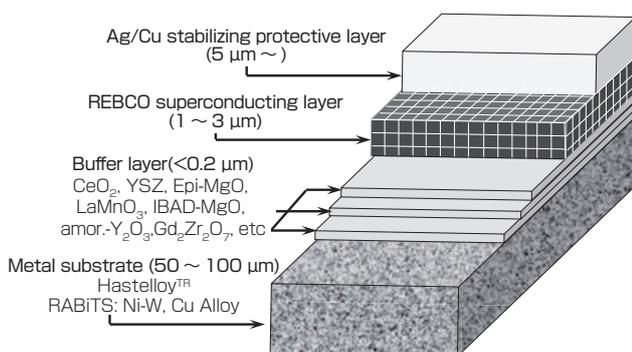
Fig. 2 Schematic diagram of REBCO tape structure
