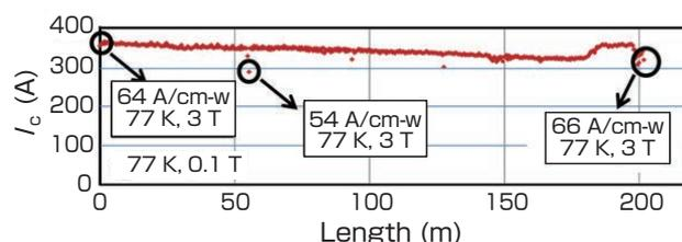
**Fig. 11 PLD long-length tape with artificial pinning center<sup>[31]</sup>**
