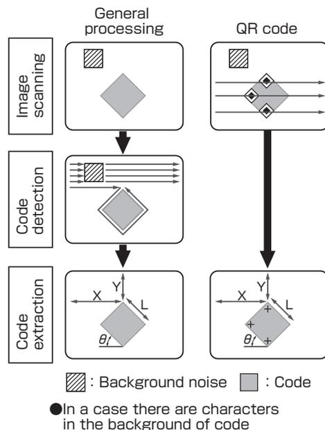
**Fig. 3 Detection processes of position and shape of code**
