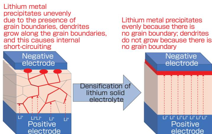
Fig. 4 Image of internal short-circuiting in all-solid-state lithium secondary battery
