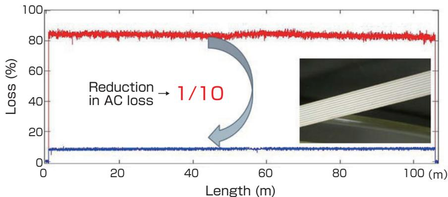
Fig. 13 Achievement of low AC loss in 100 m class tape material using scribing technology<sup>[31]</sup>
