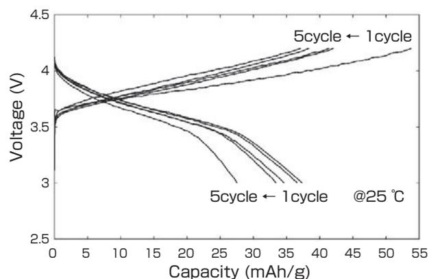
**Fig. 14 Charge/discharge property of Li / garnet-type lithium solid electrolyte / NCA all-solid-state lithium secondary battery at 25  $^{\circ}\text{C}$**
