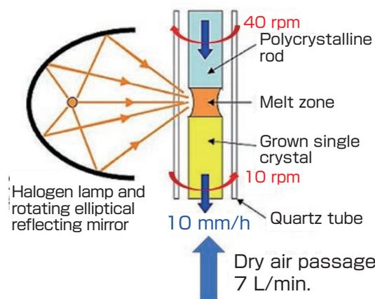
Fig. 6 Growth condition of garnet-type lithium solid electrolyte
