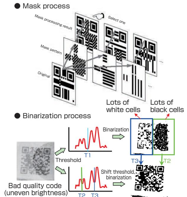
**Fig. 5 Effect of mask processing**
