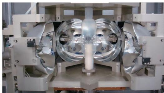
Fig. 5 Photograph of FZ melting furnace
