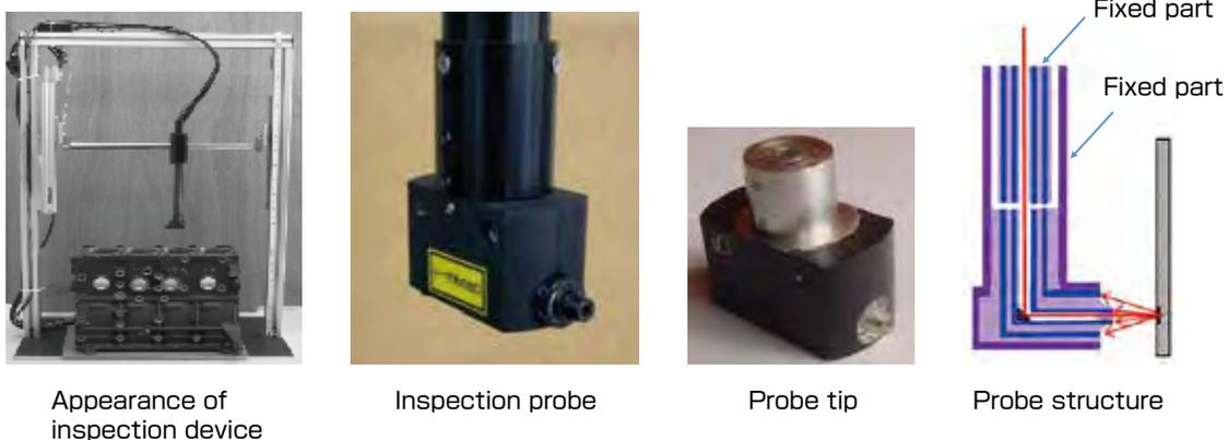
**Fig. 11 Inspection system for inner wall surfaces of machined holes**
