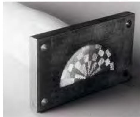
**Fig. 6 Multi-segmentation planar photodetector**
