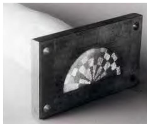
**Fig. 6 Multi-segmentation planar photodetector**
