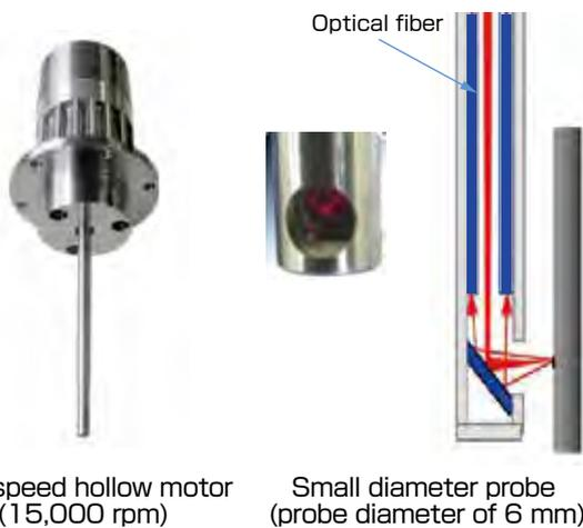
Fig. 14 Modification of inspection probe
