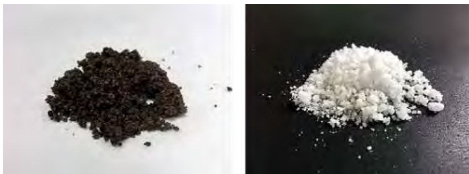
Fig. 7 Raw material molten slag (left) and synthesized silica with high specific surface area (right)
