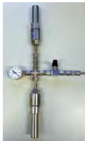
Fig. 6 Schematic diagram of reaction vessel for tetraalkoxysilane and its photograph [3]
