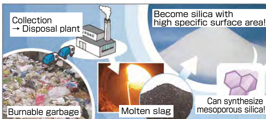
Fig. 9 Conversion of molten slag, incineration residue of burnable garbage, into high added-value material
