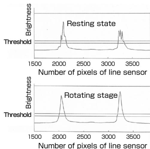
Fig. 3 Effect of line sensor rotation
