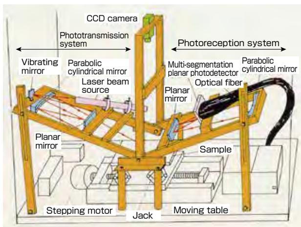
**Fig. 5 Laser defect inspection system for flat sheets**
