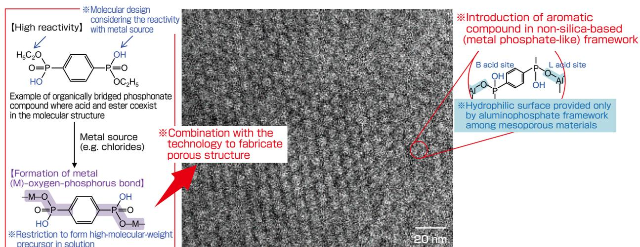
**Fig. 6** Reaction of benzene bridged phosphonate compound and metal source, which combined with the technology to fabricate mesoporous structure
