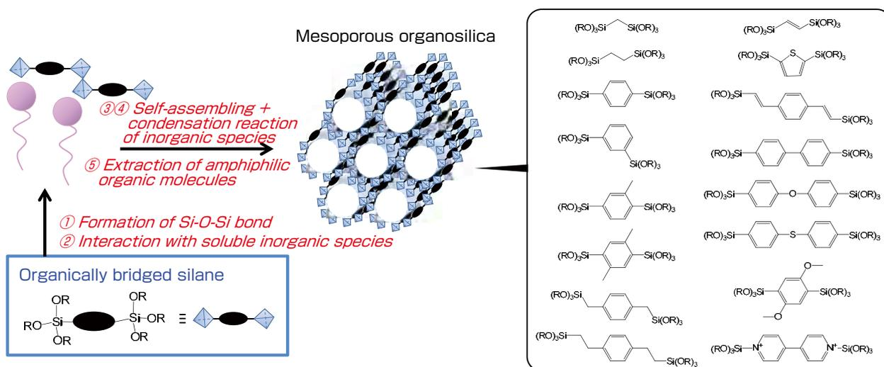
Fig. 4 Synthesis of mesoporous organosilica: Variation of organic groups (with the number of significant technologies shown in Fig. 3)
