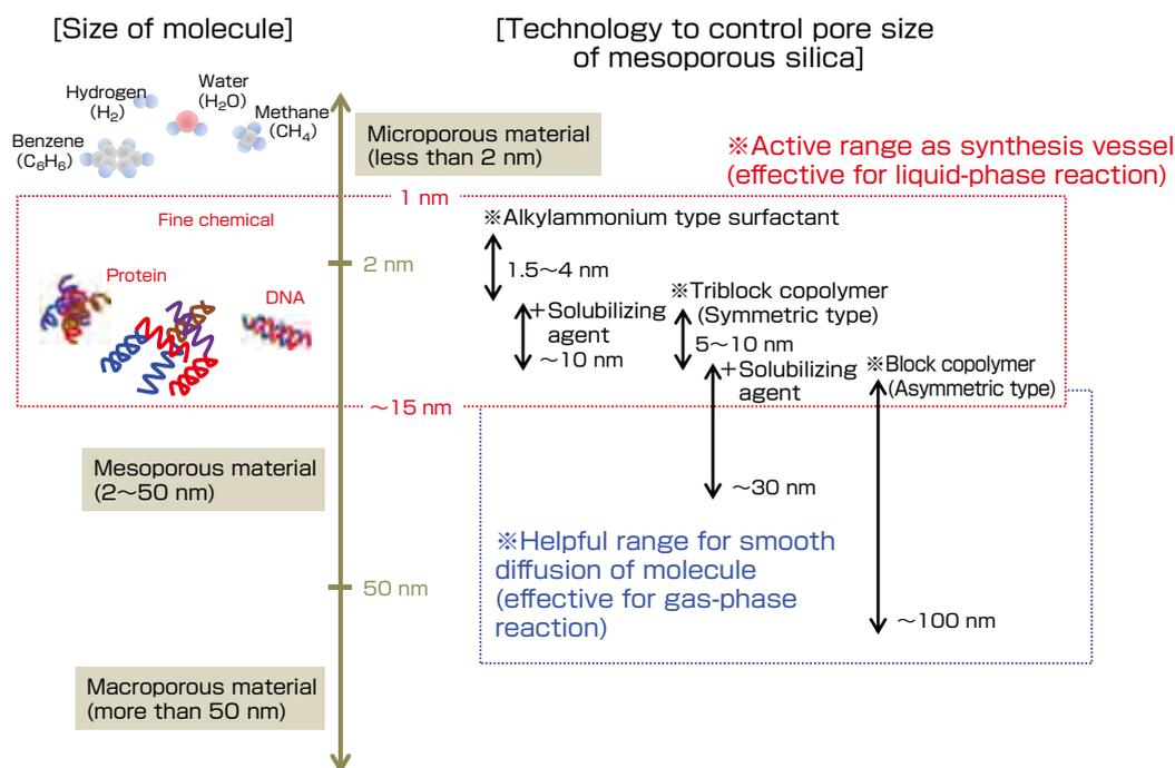
Fig. 2 Comparison between molecule size and range of pore size control of mesoporous silica
