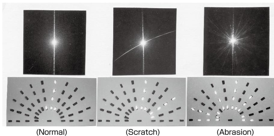
**Fig. 7 Differences in diffraction pattern by flaw types and examples of measurement by multi-segmentation planar detector**
