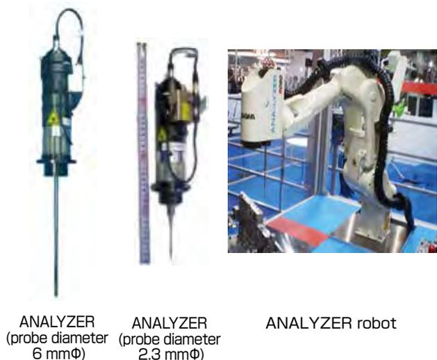
Fig. 15 Example of developed defect inspection system
