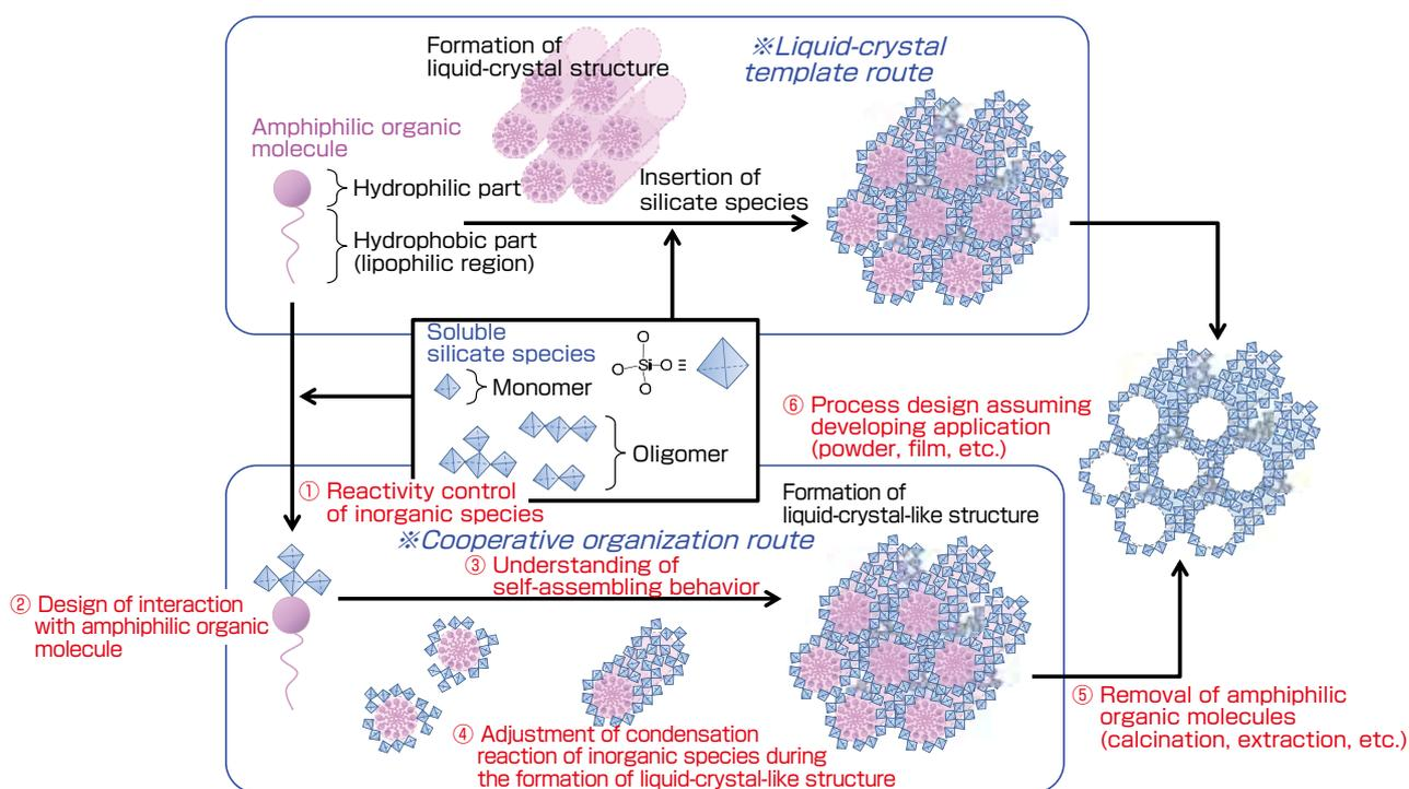
Fig. 3 Formation mechanism of mesoporous silica: Liquid-crystal templating and cooperative organization routes
