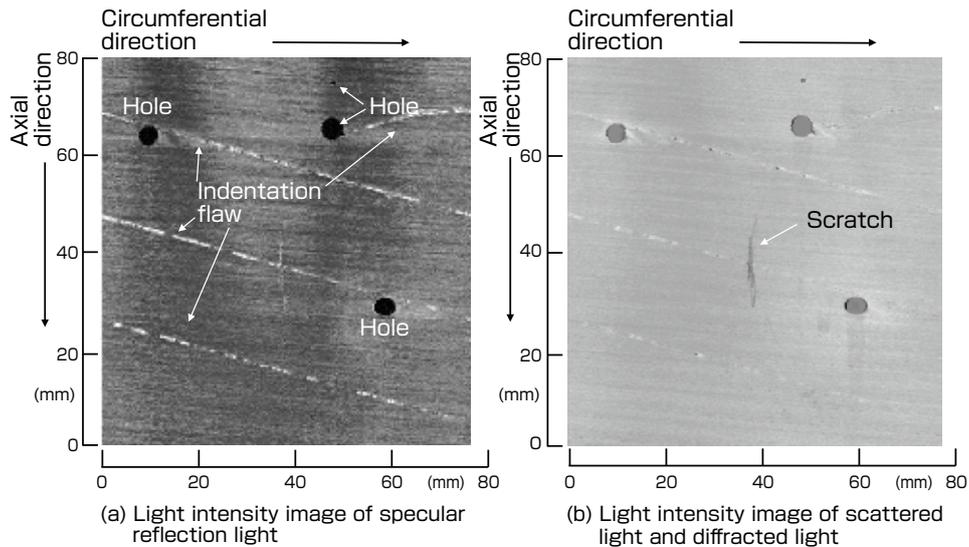
**Fig. 9** Examples of inspection images of inner wall surfaces of machined holes
