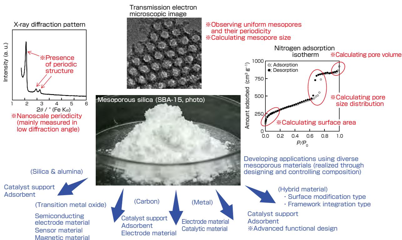
**Fig. 1 Representative analyses of mesoporous silica and examples of developing applications using diverse mesoporous materials**
