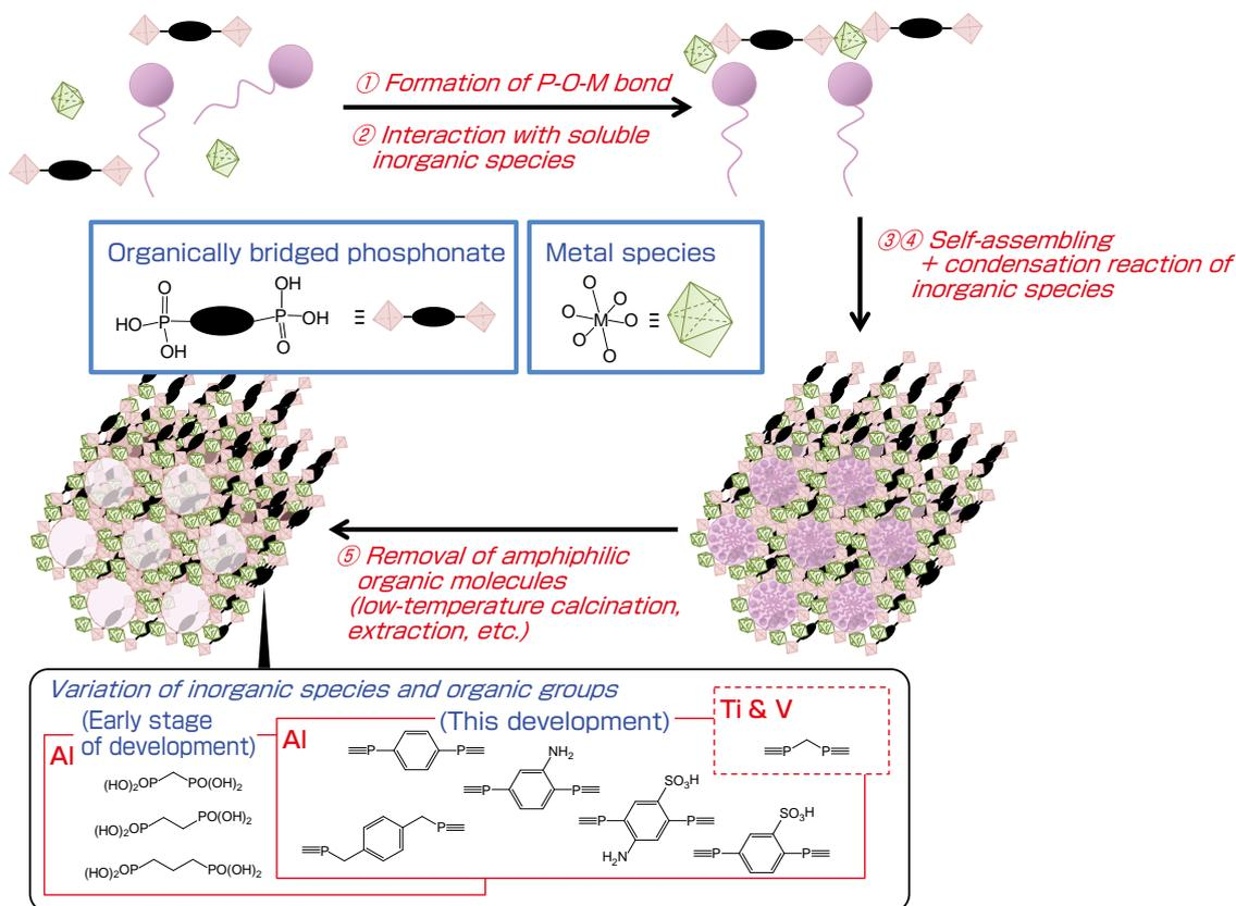
Fig. 5 Proposal of the synthesis route from organically bridged phosphonate compound, and progress in composition control technology (with the number of significant technologies shown in Fig. 3)
