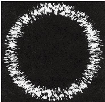
Fig. 1 Laser beam ring image by area sensor
