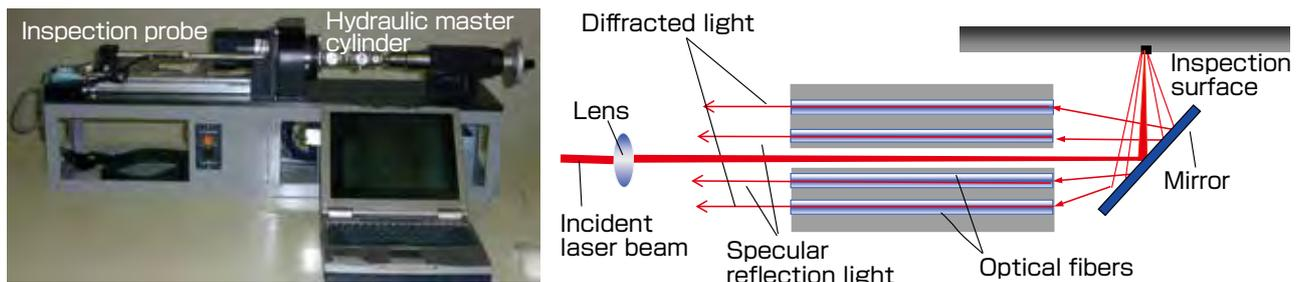
**Fig. 8 Inspection system for inner wall surfaces of machined holes**
