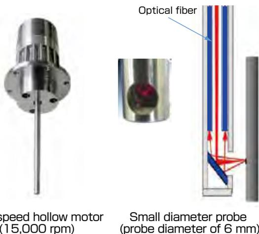
Fig. 14 Modification of inspection probe
