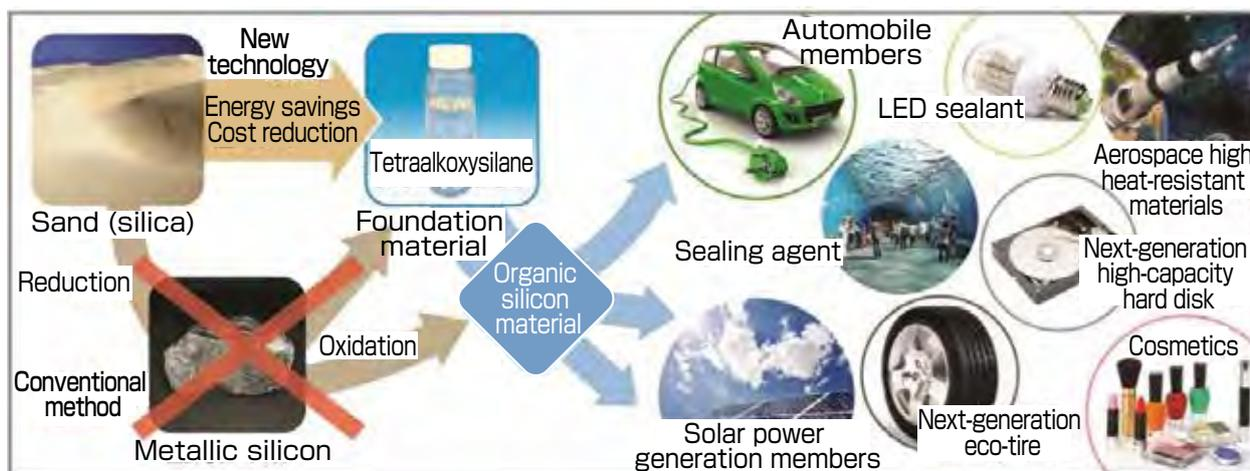
**Fig. 4 Manufacture of organic silicon material from sand (SiO<sub>2</sub>), and various product groups that contain organic silicon materials**
