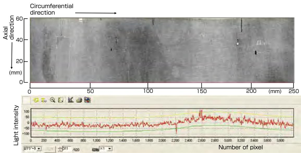
Fig. 13 Light intensity detection image of scattered light
