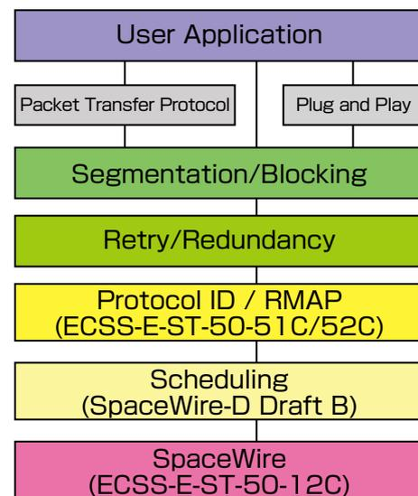
Fig. 2 Communication standard layer proposed to SpW WG from Japan<sup>[17]</sup>
