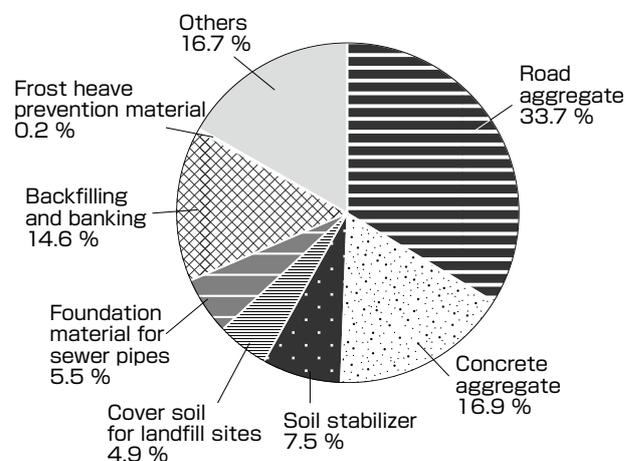
Fig. 3 Current situation of use of molten slag (from garbage and sewage sludge)<sup>[2]</sup>
