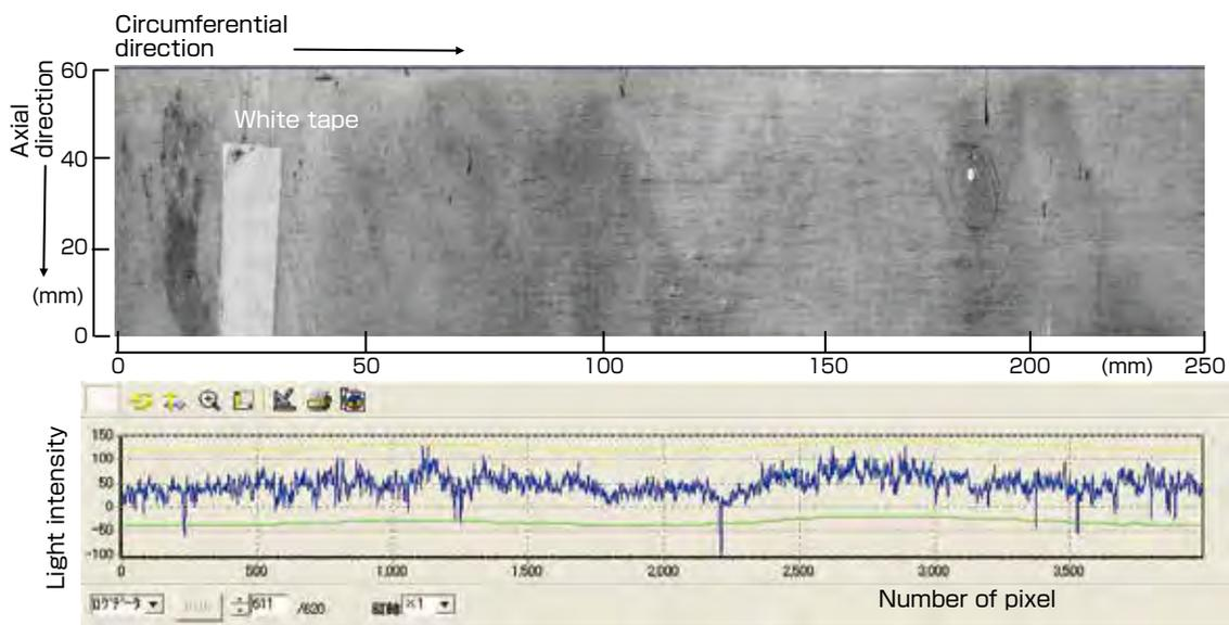
Fig. 12 Light intensity detection image of specular reflection light
