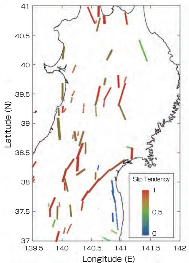
**Fig. 4 Results of activity assessment by mechanical index for active faults in Tohoku region. Regional stress field was calculated from the earthquake data before the 2011 off the Pacific Coast of Tohoku Earthquake (East Japan Earthquake) ([10] was partially revised).**
