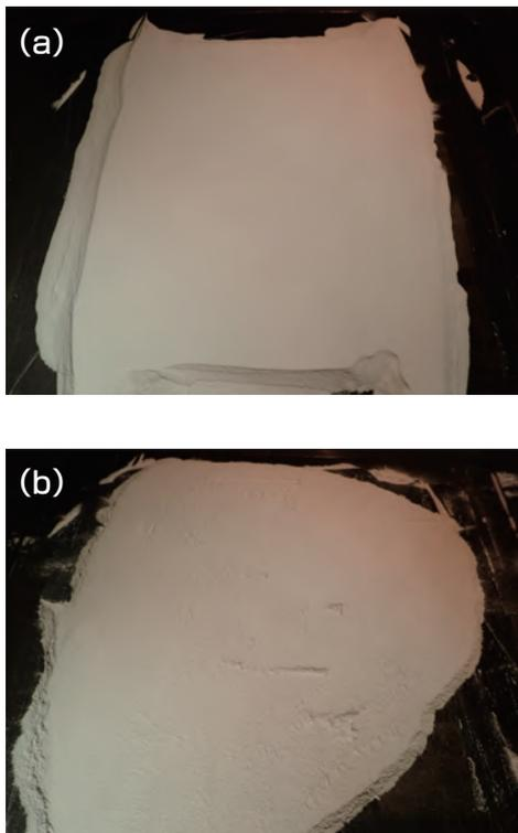
Fig. 6 Preliminary powder test for lamination, (a) Smooth surface with flowable powder, (b) Dimples and cracks with less flowable powder
