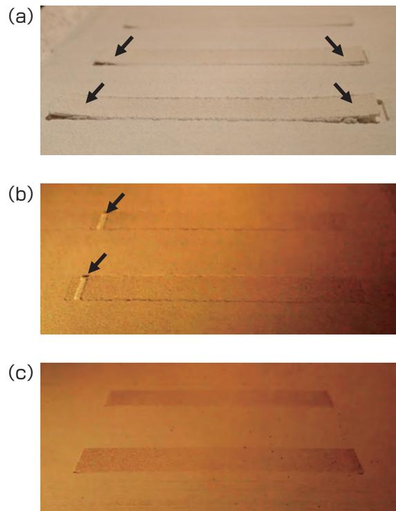
**Fig. 7 (a) Warping observed in a green body with nylon-based binder, (b) Sliding of a green body and formation of a gap, (c) Successful formation of a green body embedded in powder. The body is rectangular-shaped with 7 mm width and 50 mm length.**
