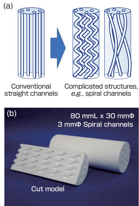
Fig. 10 (a) Conventional water-purification ceramic filter has unidirectional straight channels, while the AM techniques enable more complicated channels, *e.g.*, spiral ones. (b) an alumina filter model produced by PLM, containing spiral channels of 3 mm diameter whose traces are observed in the cut model
