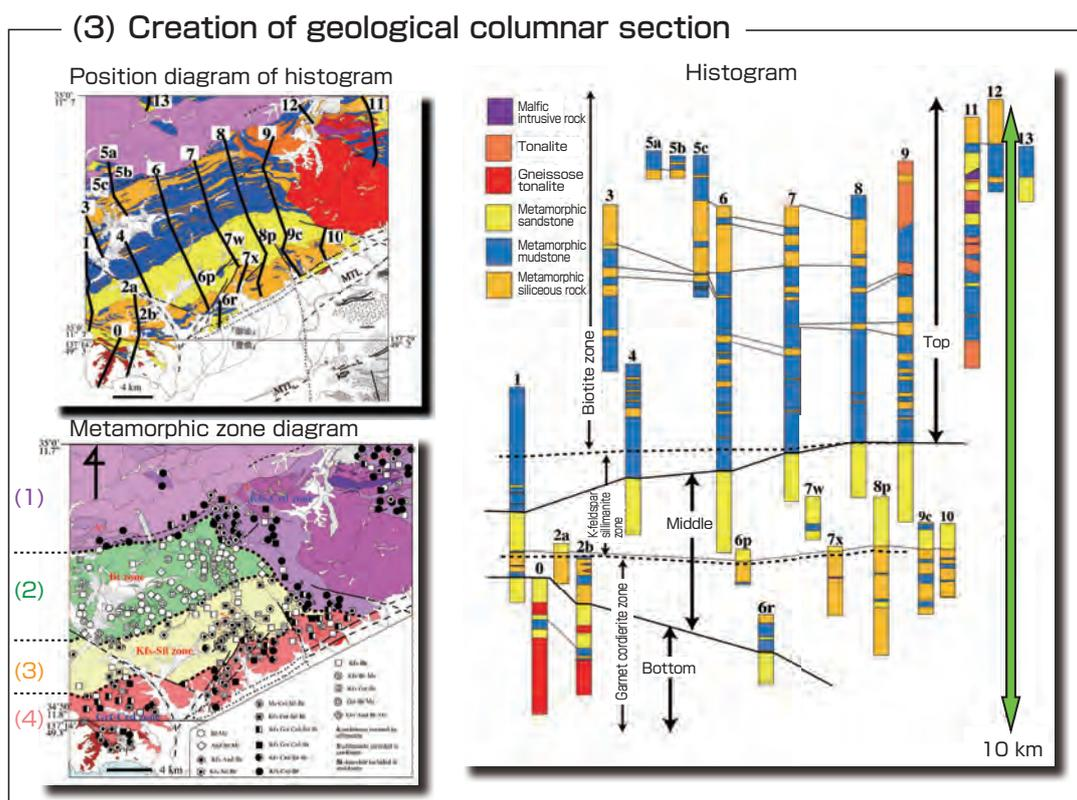
**Fig. 13 Example of geological columnar section created in field survey (quadrangle geological map “Goyu”)<sup>[7]</sup>**
