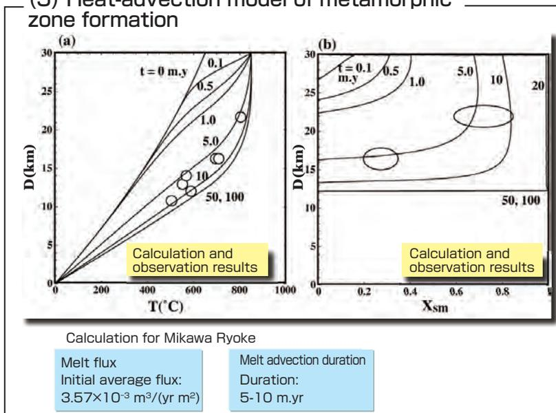
**Fig. 15 Example of heat-advection model for formation of metamorphic zone (Ryoke metamorphic rock, Mikawa plateau) in laboratory research<sup>[8]</sup>**
