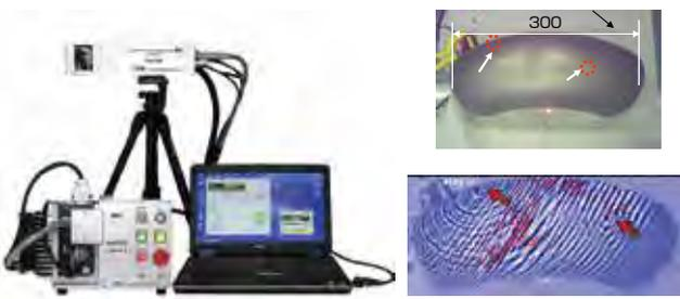
**Fig. 1 Laser ultrasonic visualization inspector and an example of visualized image**
