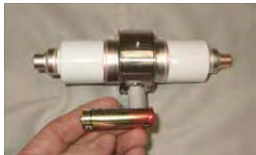
Fig. 15 Cold cathode X-ray tube equipped with carbon nanostructure cold cathode electron source
