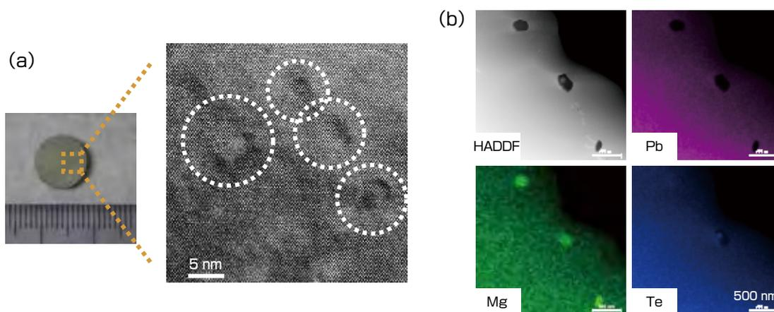
**Fig. 5 (a) Typical appearance and high-magnification transmission electron microscopy image<sup>[12]</sup> and (b) energy-dispersive X-ray elemental mapping of the sintered compact of p-type  $(\text{Pb}_{0.94}\text{Mg}_{0.02}\text{Na}_{0.04})\text{Te}$ .<sup>[12]</sup>**
