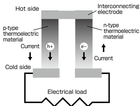
Fig. b Thermoelectric module made from one couple of p- and n-type thermoelectric materials
