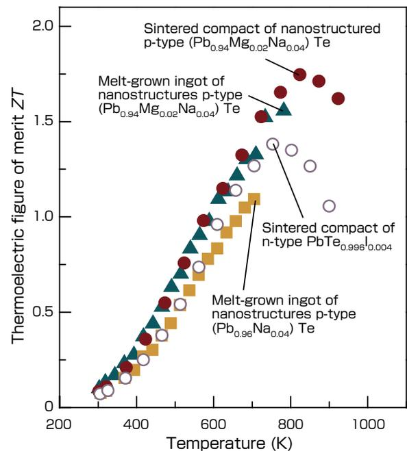
**Fig. 4** Temperature dependence of the thermoelectric figure of merit *ZT* for the melt-grown ingots and sintered compacts of p- and n-type PbTe<sup>[10][12]</sup>
