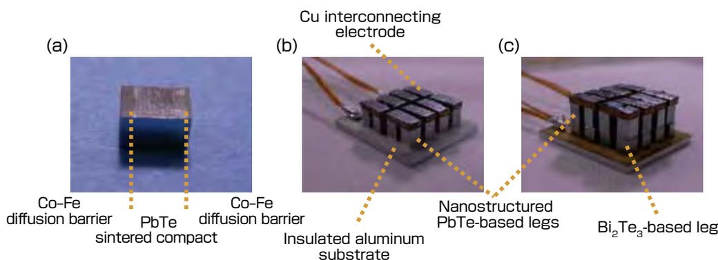
**Fig. 6 Nanostructured PbTe-based (a) thermoelectric element, (b) single-stage thermoelectric module, and (c) two-stage (segmented) thermoelectric module using  $\text{Bi}_2\text{Te}_3$ <sup>[12]</sup>**
