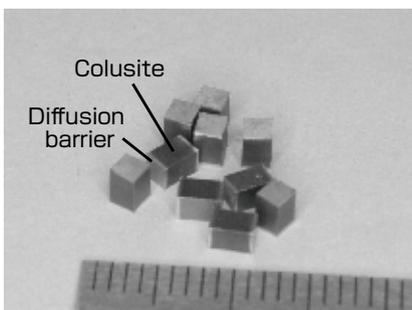
**Fig. 9 Colusite-based thermoelectric elements. Au-based diffusion barriers are formed on both sides.**
