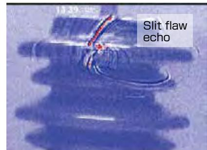
Fig. 10 Insulator with cracks
