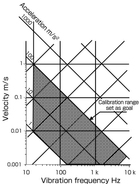
**Fig. 5 Relationship of displacement, velocity, and acceleration in sine wave vibration and their calibration range**
