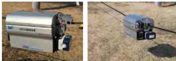
Scene of self-propulsion test on power line
