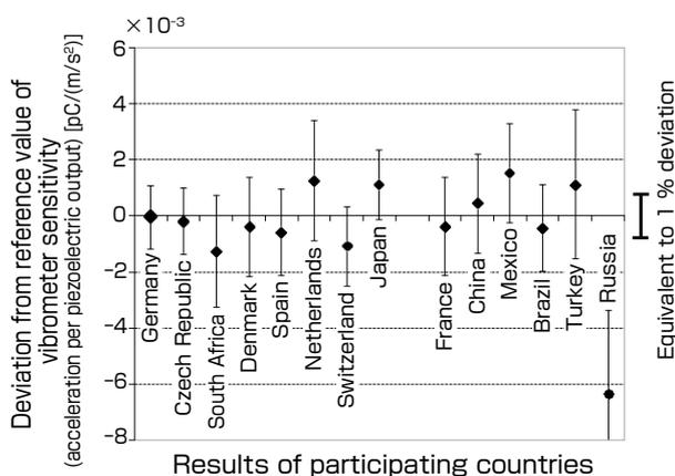
Fig. 12 An example of the results of the second international comparison for vibrometer calibration
