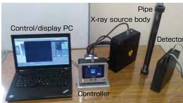
Fig. 20 Compact X-ray inspector for pipes
