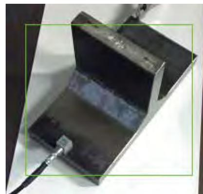
**Fig. 6 T-shaped welded joint (defect in welded corner part)**
