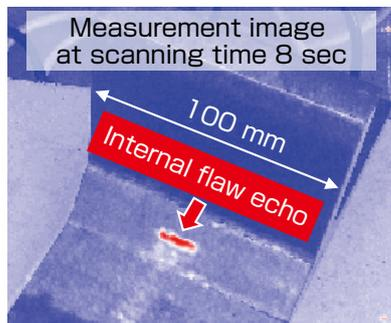
② Scanning rate 5,000 Hz; scanning pitch 0.8 mm
