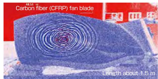
**Fig. 9 Ultrasound propagation image of the CFRP aircraft fan blade**
