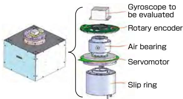
**Fig. 21 Gyro calibration device**
