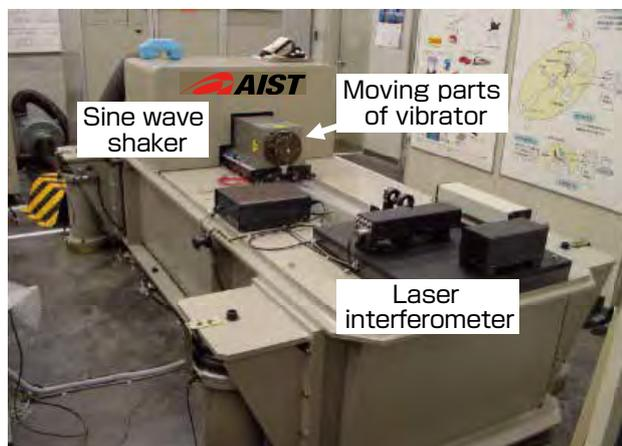
**Fig. 13** Developed calibration device for vibrometer with minimum frequency 0.1 Hz
