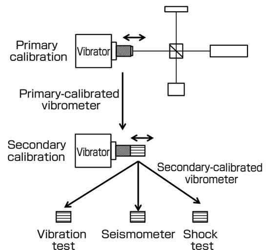
**Fig. 4** Traceability in vibrometer calibration
