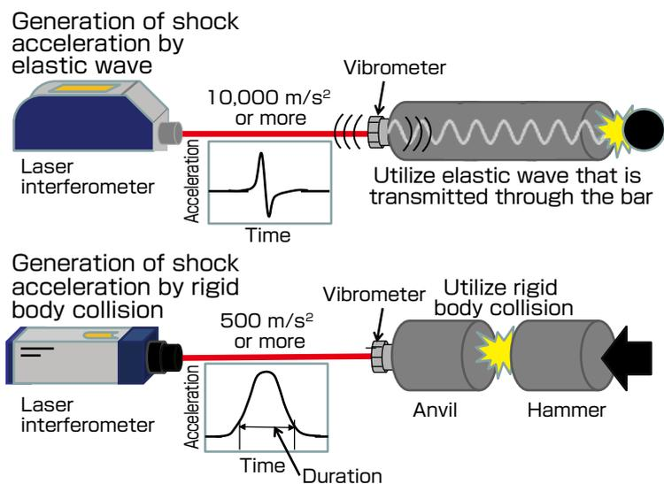
Fig. 16 Generation of shock acceleration and calibration of vibrometer
