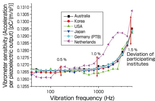
**Fig. 9 An example of the results of the first international comparison for vibrometer calibration**
