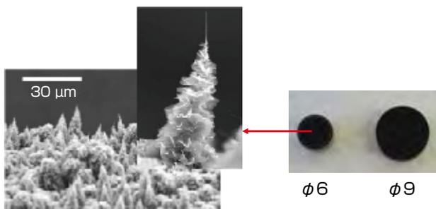
Fig. 14 Carbon nanostructure (left) and cold cathode electron source (right)
