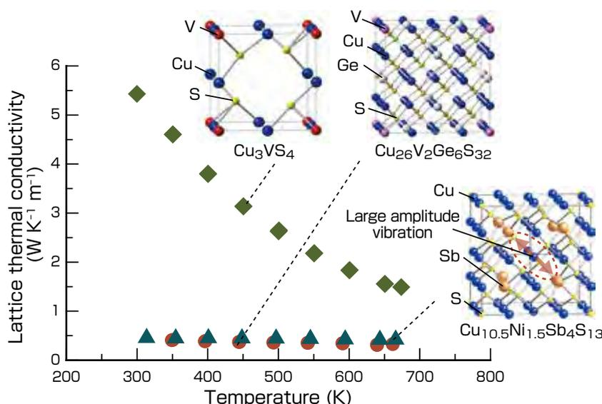
**Fig. 8** Temperature dependence of thermal conductivity for tetrahedrite  $\text{Cu}_{10.5}\text{Ni}_{1.5}\text{Sb}_4\text{S}_{13}$ ,<sup>[26]</sup> colusites  $\text{Cu}_{26}\text{V}_2\text{Ge}_6\text{S}_{32}$ ,<sup>[29]</sup> and sylvanite  $\text{Cu}_3\text{VS}_4$ ,<sup>[29]</sup> along with their crystal structures.
