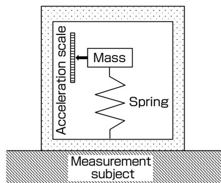
Fig. 1 Seismic system vibrometer
