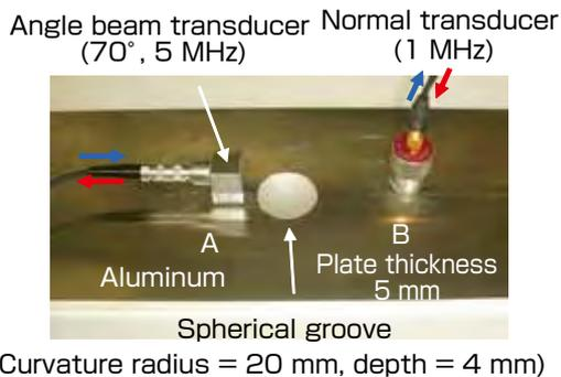
**Fig. 2 Reciprocity of ultrasound propagation**
