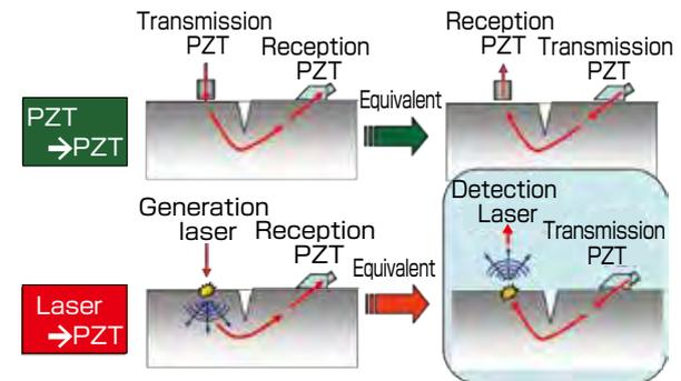
**Fig. 3 Comparison of reciprocities of PZT-PZT transceiver system and laser-PZT transceiver system**
