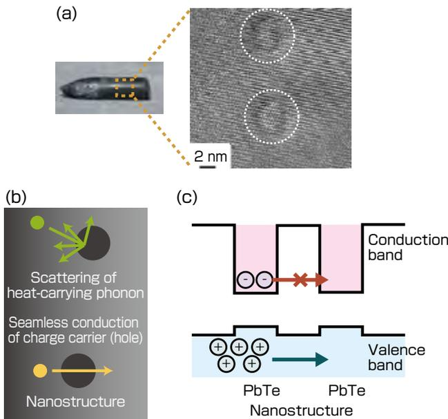
**Fig. 3** (a) Typical photograph and high-magnification transmission electron microscopy image of the melt-grown ingot of p-type (Pb<sub>0.94</sub>Mg<sub>0.02</sub>Na<sub>0.04</sub>)Te,<sup>[10]</sup> (b) conceptual diagram of the enhancement in the thermoelectric figure of merit *ZT* through nanostructuring, and (c) expected band alignment of nanostructure in the p-type PbTe matrix.<sup>[11]</sup>
