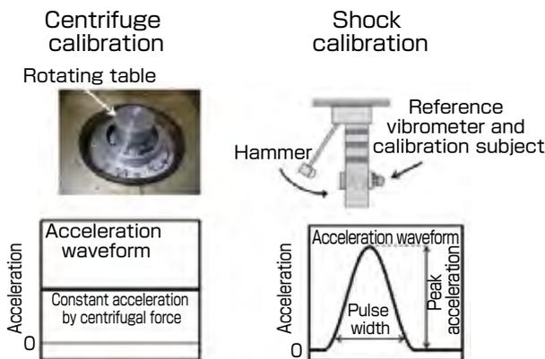
**Fig. 19 Calibration method for large amplitude acceleration used in industry**
