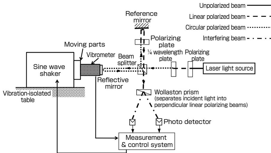
**Fig. 6 Developed laser interferometer**
