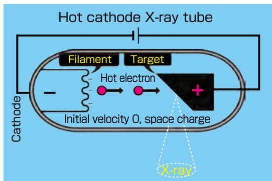
Fig. 16 Internal structure of the Hot cathode X-ray tube
