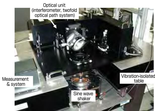
Fig. 11 Developed calibration device for vibrometer up to 10 kHz
