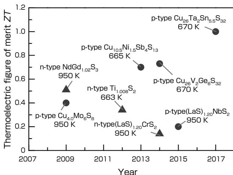
**Fig. 7 Thermoelectric sulfides developed in this study:**
