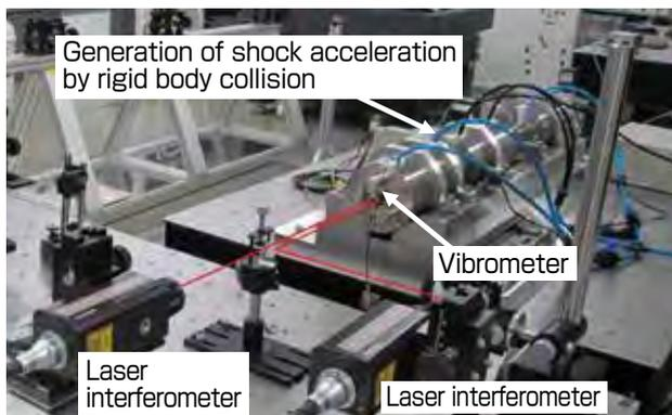
Fig. 17 Developed shock calibration device
