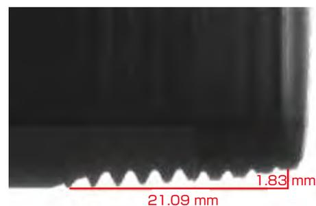
Fig. 21 Example of display of pipe size
