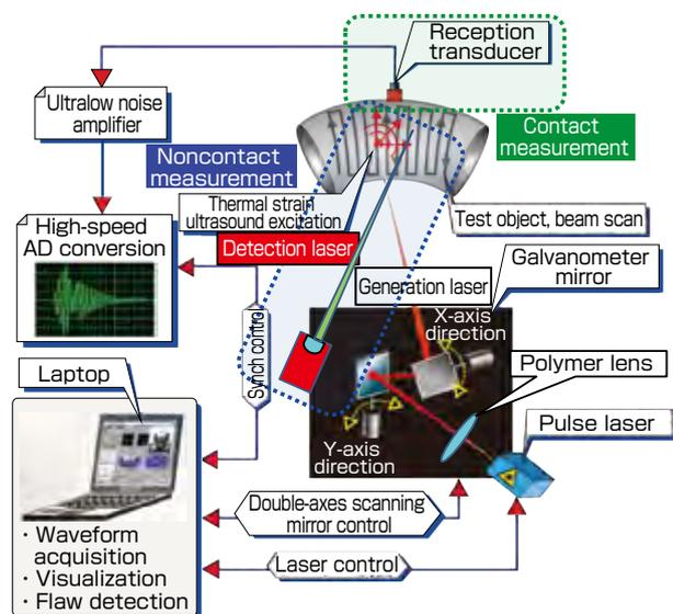
**Fig. 4 Configuration of the laser ultrasonic visualization inspector (LUVI)**
