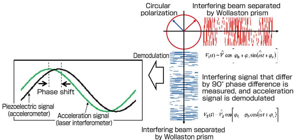
**Fig. 7 Detected interfering signal**
