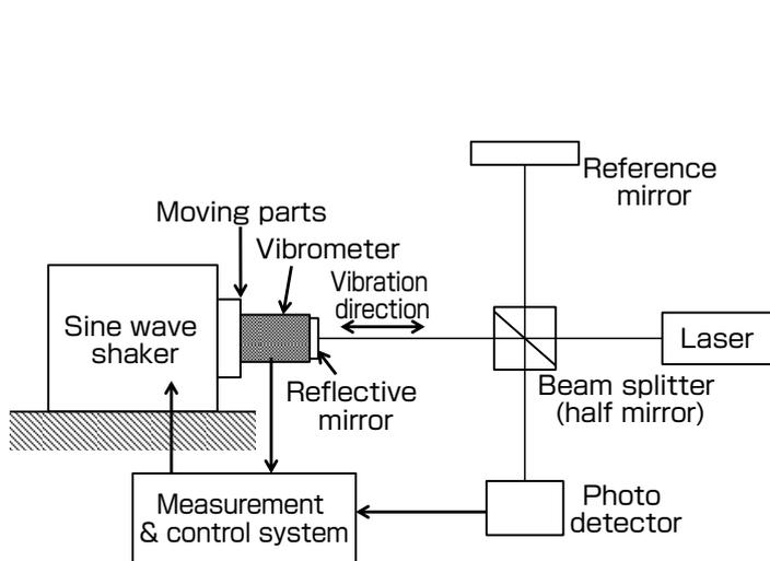
**Fig. 3** Vibrometer calibration device
