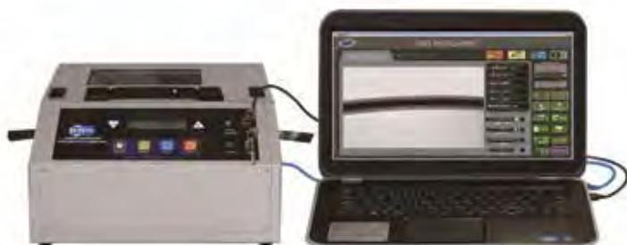
Fig. 22 Compact X-ray inspector for power lines
