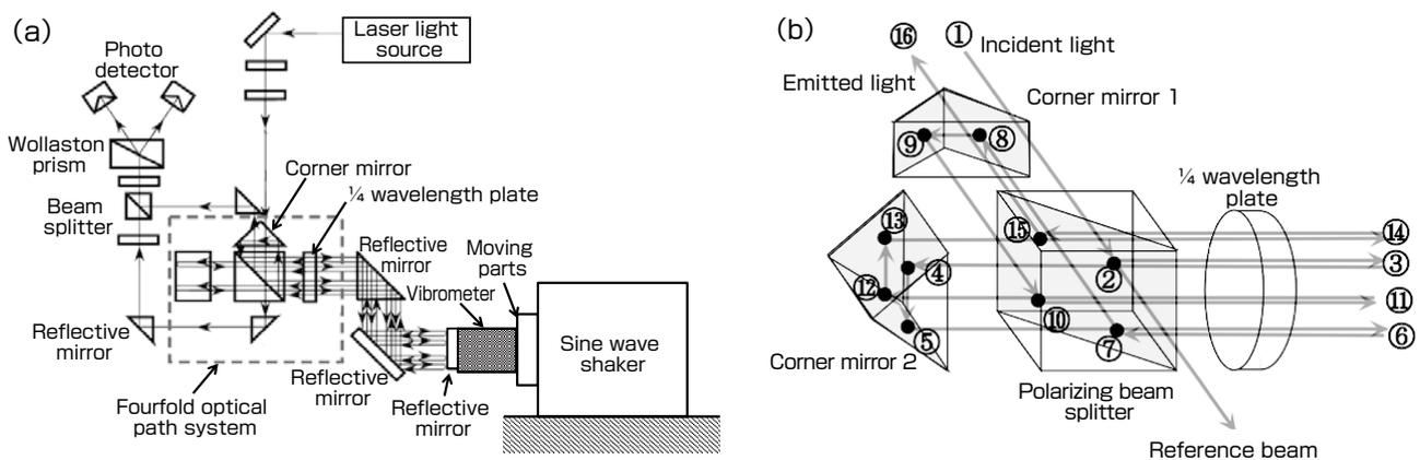
**Fig. 10 Configuration of the developed laser interferometer and its optical path arrangement**
