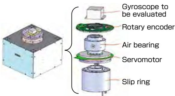
**Fig. 21 Gyro calibration device**
