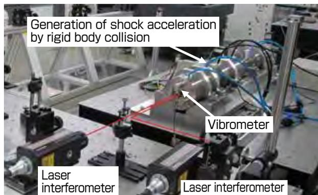
Fig. 17 Developed shock calibration device
