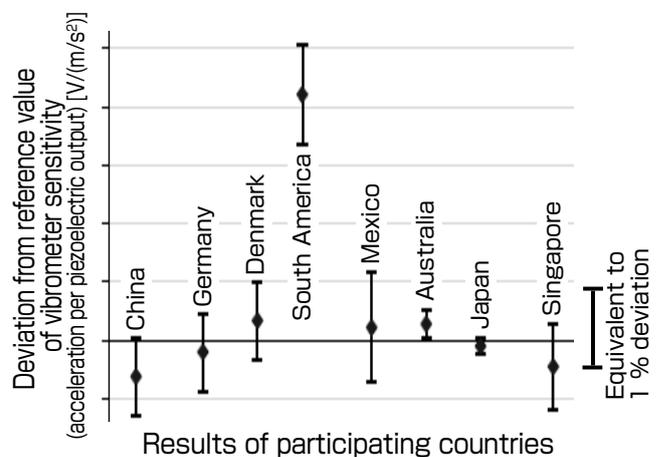
**Fig. 14** An example of the results of the third international comparison for vibrometer calibration
