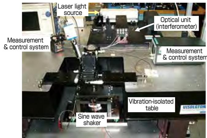
**Fig. 8 Developed calibration device for vibrometer up to 5 kHz**
