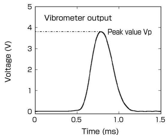
Fig. 18 Acceleration waveform obtained from the shock calibration device and output from the vibrometer
