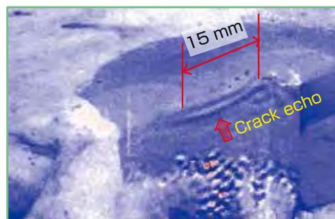
Fig. 13 Fatigue crack echo of the welded part of steel bridge
