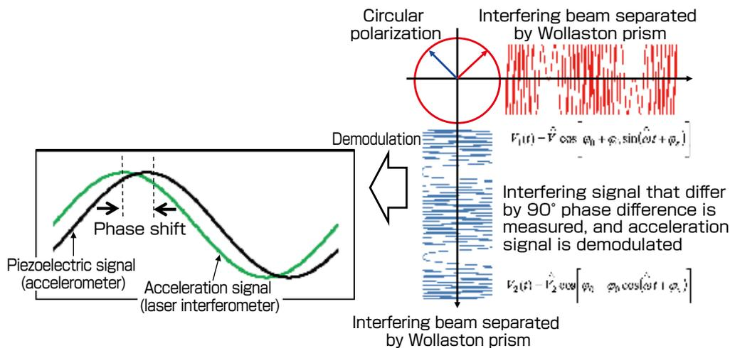
Fig. 7 Detected interfering signal
