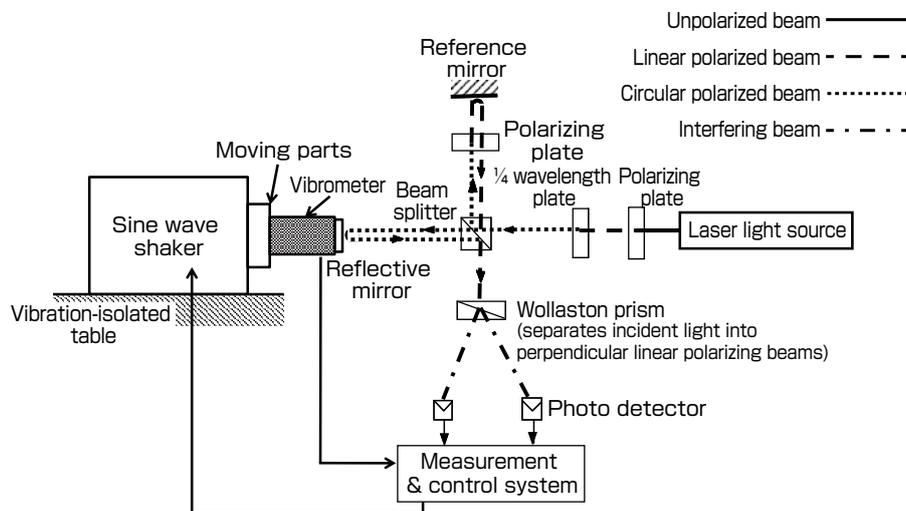
**Fig. 6 Developed laser interferometer**
