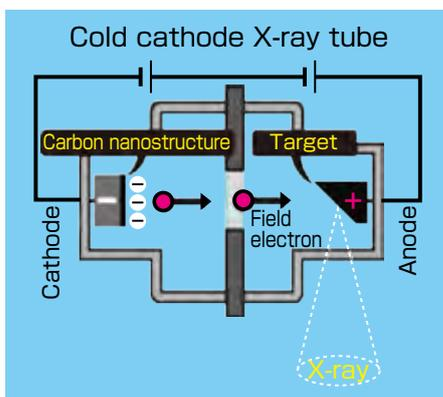
Fig. 17 Internal structure of the cold cathode X-ray tube
