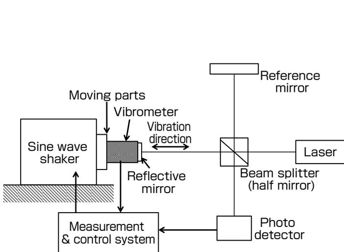
**Fig. 3** Vibrometer calibration device
