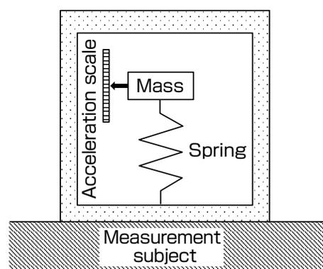
Fig. 1 Seismic system vibrometer
