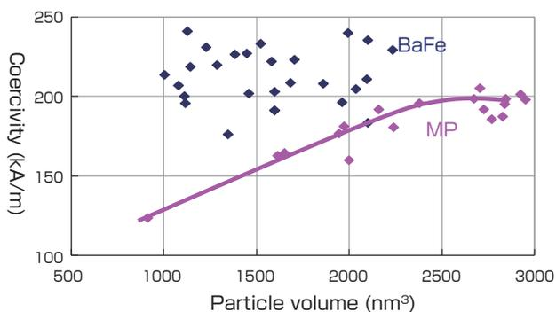
**Fig. 6 Particle volume and coercivity of the magnetic material**
