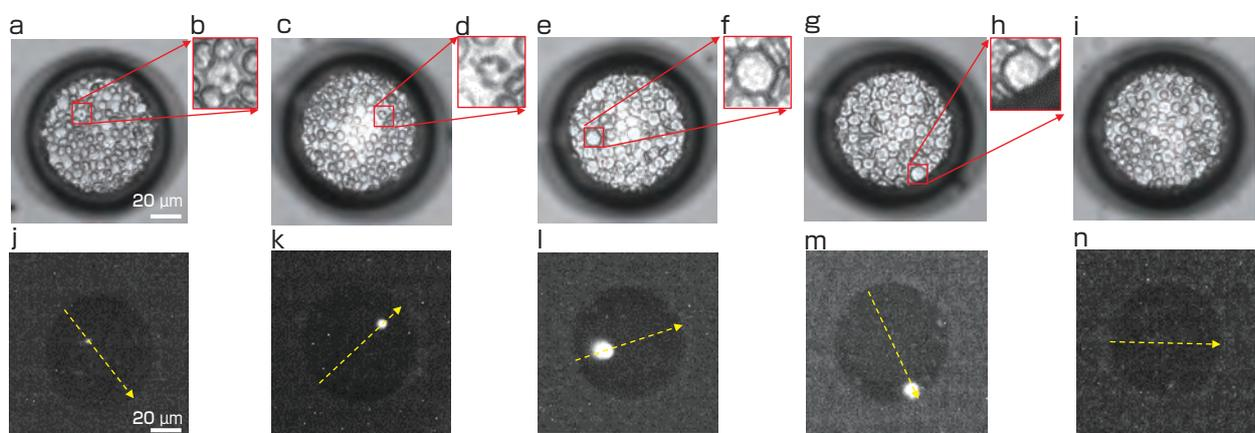
**Fig. 3 Separation of the leucocytes and infected erythrocytes in the microchamber**
