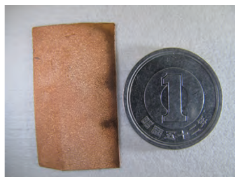
CNT-Cu composite material possessing 100-times higher current carrying capacity, 40% lower density, and a lower resistivity at elevated temperatures than copper, while also exhibiting the same coefficient of thermal expansion as silicon
