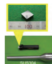
Rare metal free TiC-FeAl cutting tool and cut stainless bar
