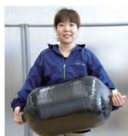
Lightweight hydrogen tank with hydrogen barrier clay-layer
