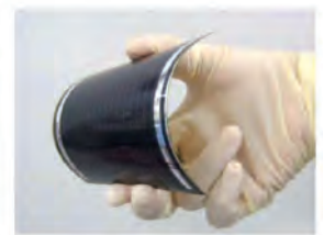
High efficiency (15.9 %) flexible CIGS sub-module fabricated on stainless substrate
