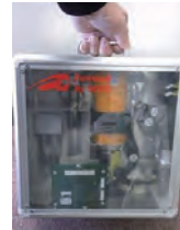
Prototype Portable SOFC System (Max. Power 200W)
