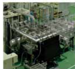
The G5 size (1.1 mx1.4 m) CVD machine development activity by collaboration of consortium companies.
