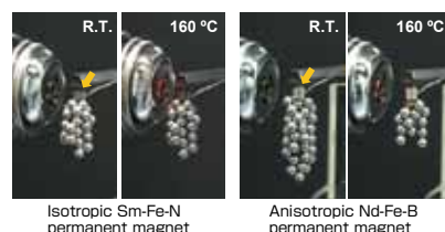
Comparison of heat resistance between the developed isotropic Sm-Fe-N magnet and the conventional anisotropic Nd-Fe-B magnet (change in the number of magnetic-attracted iron balls on each magnet by heating).
