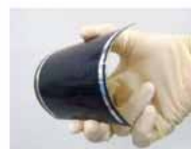
High efficiency (15.9 %) flexible CIGS sub-module fabricated on stainless substrate.
