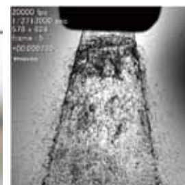
High speed camera image of coating spray pattern using supercritical carbon dioxide
