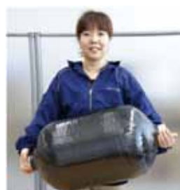
Lightweight hydrogen tank with hydrogen barrier clay-layer
